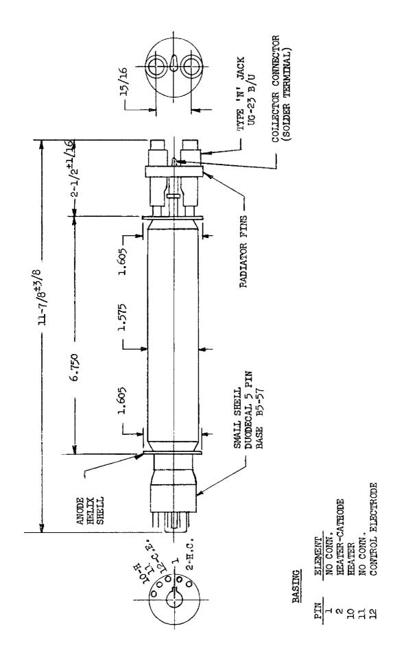
TRAVELING WAVE TUBE TYPES F-6658, F-6868, and F-6996
