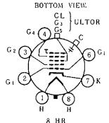
Pin 7: Cathode Pin 8: Heater
