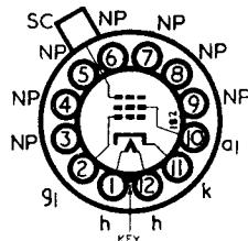
The BRIMAR C21TM is a rectangular 90° deflection angle teletube with magnetic focus, a tetrode gun incorporating an ion trap, aluminized screen and external conductive coating. The screen colour is white, with a grey glass faceplate with a transmission of approximately 70 per cent.
