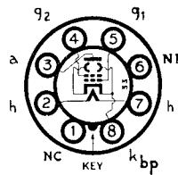
The BRIMAR type 12A6 is an indirectly heated output beam tetrode of high efficiency for use in car radio or A.C./D.C. receivers, where the supply exceeds 110 volts.
