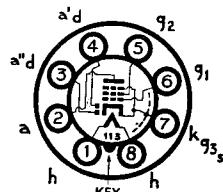
The BRIMAR type 7R7 is a multiple valve of "all glass" construction designed for simultaneous operation as detector and I.F. or L.F. amplifier in radio receivers. The pentode section has semi-vari-mu characteristics and A.V.C. may be applied.
