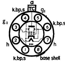
The BRIMAR 6146 is an octal based beam tetrode for use as an R.F. power amplifier up to 175 Mc/s or as an A.F. power amplifier or modulator.
