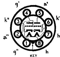
BRIMAR type 13D1 has been specially designed for use in aircraft and Industrial equipment where reliability is of importance. It supersedes type 25SN7GT and is a direct replacement for it. Except for the heater rating the characteristics are nominally the same as for the type 6SN7GT.
