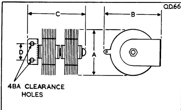
Note:—The two centre tags must be connected together before rectifier is put into operation.
