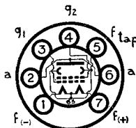
BRIMAR type 3S4 completes the range of miniature valves for use in battery receivers and compact portable equipment. The filament is in two sections which may be series or parallel connected. When series connected type 3S4 may be used in conjunction with other valves in the range and the filament operated from a high voltage source where the current is limited to 50 mA. When parallel connected this valve has identical characteristics to BRIMAR type 1S4 which it supersedes.
