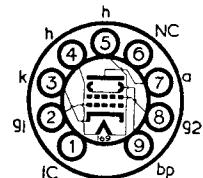
The BRIMAR type 6BW6 is a B9A (Noval) based output beam tetrode, the characteristics and ratings of which are identical to those of the 6V6G/GT. It is suitable for R.F. application up to frequencies of the order of 150 Mc/s.
