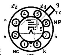
Note.—Pin 1 connected to metal shell.
