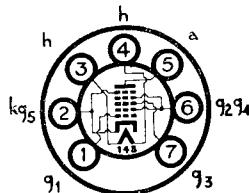
The BRIMAR 12AD6 is a miniature frequency changer for use in car radio receivers to operate directly from the 12-volt battery without the use of a vibrator H.T. system. It is designed to operate over the range of voltage variations normally encountered with car batteries.
