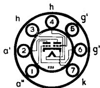
The BRIMAR 6J6 is a miniature double triode with a common cathode and may be used as a mixer or R.F. oscillator and in the latter application will produce a power output of 3.5 watts at frequencies up to 50 Mc/s. It is useful as a mixer up to 600 Mc/s.
