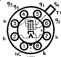
Note.—Type 6A8GT has Pin 1 connected to metal shell.
