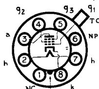
Note.—Type 6K7GT has Pin 1 connected to metal shell.
