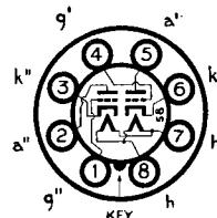
The BRIMAR type 6SN7GT is an indirectly heated valve comprising two general purpose triodes in one envelope. With the exception of the heaters, the connections to each assembly are brought out to separate base pins. Type 6SN7GT may be used as oscillator, L.F. amplifier, phase inverter, etc., or the two units may be connected in cascade to give a high overall gain. The operating characteristics of each section are identical to those of type 6J5GT.
