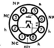
The BRIMAR type 35Z4GT is an indirectly heated half-wave rectifier for use in A.C./D.C. equipment where low heater current drain is of importance.
