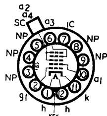
Rectangular Wide Angle Deflection, Electrostatic Focus Teletube, with Ion trap,
