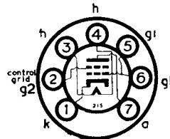
The BRIMAR 12K5 is a miniature tetrode with a space charge grid,  $g_1$ , the control grid being  $g_2$ . The valve is intended for use as a driver stage in A.F. applications in car radio receivers and will operate directly from the 12-volt battery without the use of vibrator H.T. system. It is designed to operate over the range of voltage variation normally encountered with car batteries.
