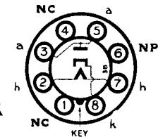
The BRIMAR type 25Z4G is an indirectly heated half-wave rectifier for use in A.C./D.C. equipment. It is designed to replace type 25Z6G where this valve is used in half-wave application.
