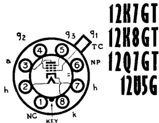
Note.—Pin 1 connected to metal shell.
