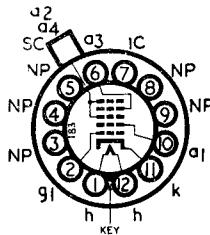
The BRIMAR C21SM is a rectangular 90° deflection angle teletube with electrostatic focus, an aluminized screen and external conductive coating. The screen colour is white with a grey glass faceplate with a transmission of approximately 70 per cent.
