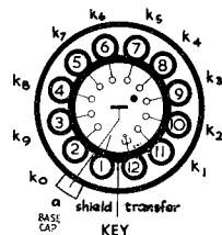
The G10/24IE is a single-ended cold-cathode unidirectional gas-filled counter and distributor tube. It has ten cathodes which are used to indicate the number of the count, either visually at low speeds or by means of the voltage developed across the cathode load at high speeds. It is capable of counting pulses at repetition speeds from approximately 0 up to 20 kc/s.
