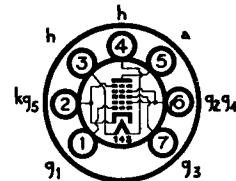
The BRIMAR 7032 is a miniature heptode with short grid base characteristics on grid 1 and grid 3. It is of Trustworthy construction and is intended for use in computers as a gating valve or in similar applications. The cathode has been designed to give good life and reliability when used for long periods under cut-off conditions.
