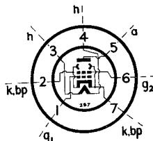
The BRIMAR F/7001 is a miniature beam tetrode intended primarily for use as an R.F. amplifier up to 50 Mc/s in mobile equipment. It is a Trustworthy valve and has been designed for use under adverse conditions of vibration and shock.
