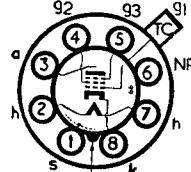
Note.—Type 6J7GT, has Pin 1 connected to metal shell.
