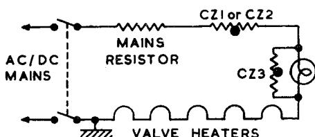
When a CZ1 or CZ2 Brimistor is fitted as a surge suppressor the pilot lamp may often be run safely at a higher temperature. The shunt resistor across the lamp may be removed and a type CZ3 Brimistor wired in place of it. Should the lamp eventually fail, the CZ3 will warm up quickly and the set will continue to operate at full efficiency.
