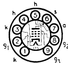
The BRIMAR 6BW7 is a high slope R.F. pentode designed for use in the R.F. Frequency Changer, I.F. and Video stages of television receivers. The valve features high mutual conductance together with a high R.F. input impedance, achieved by the use of two cathode connections. Type 6BW7 will operate from a 180 or 250 volt H.T. rail, making it suitable for both AC/DC and AC operated receivers.
