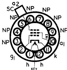
Rectangular Wide Angle Deflection Teletube with tetrode gun, ion trap, aluminized screen and external conductive coating.
