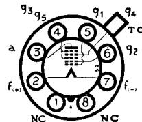
Note.—Type IA7GT has Pin 1 connected to metal shell.
