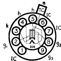
The BRIMAR PL81/21A6 is designed for operation as the line time-base output valve in A.C./D.C. television receivers. Used in conjunction with a booster diode it is suitable for the scanning of wide angle ( $70^\circ$ ) cathode ray tubes from low H.T. rail voltages.
