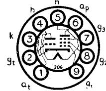
The BRIMAR ECL80/6AB8 is a triode pentode with a common cathode designed for use in the frame time base circuits of television receivers. The triode may be used as frame blocking oscillator and the pentode in the frame output stage. The triode may also be used as a line time base generator or an A.F. voltage amplifier and the pentode as a sync. separator or an audio output valve. It is suitable for use in A.C. or A.C./D.C. receivers.
