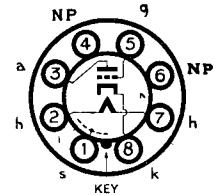
The BRIMAR type 6C5G is a small triode suitable for use as detector, oscillator or L.F. amplifier valve.
