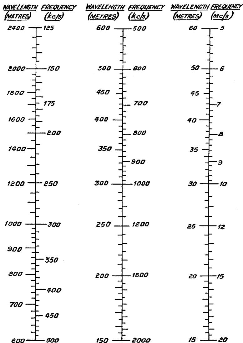
The velocity of radio waves in air is approximately 300,000 kilometres/sec.
