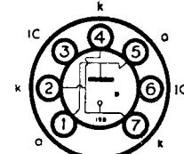
The G55/1K is a miniature cold-cathode, gas-filled, voltage-stabiliser for use in industrial and radio equipment where a stable source of voltage is required. The noteworthy feature of this valve is the relatively low maintaining voltage of 55 volts.
