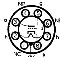
Note.—Type 6J5GT has Pin 1 connected to metal shell.
