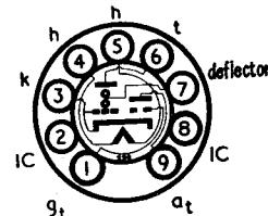
The BRIMAR EM840 is a novel based tuning indicator with the luminous target deposited on the glass itself in the form of a vertical strip. Each end of this strip is luminous and on the application of a control voltage, the luminous areas extend inwards to the centre from the ends.
