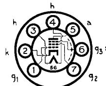
The BRIMAR type 9D6 is an indirectly heated vari-mu R.F. pentode of "all glass" construction, fitted with a miniature type base. Owing to its relatively high slope and small physical size, type 9D6 is particularly suitable for use in the R.F. and I.F. stages of compact radio equipment.
