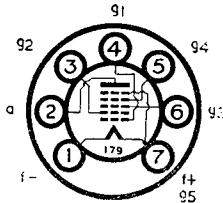
The BRIMAR 1AC6 is a new battery heptode frequency changer featuring improved short-wave performance and reduction in H.T. current consumption compared with type 1R5. The provision of separate connections for the oscillator anode and screen grid allow the use of conventional oscillator circuits and a much improved oscillator performance. As a self oscillating frequency changer it operates uniformly up to 30 Mc/s.
