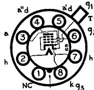
Note.—Type 6B8GT has Pin 1 connected to metal shell.
