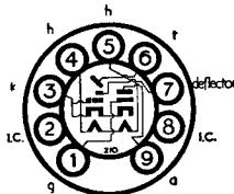
BRIMAR type EM85 is a Noval based " Magic Eye " with the screen viewed through the side of the bulb. The display is green with a dark fan-shaped area in the centre.
