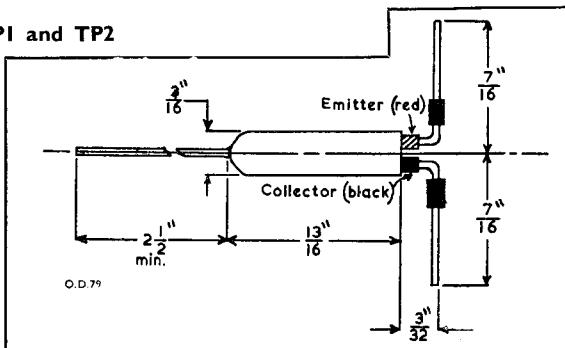
The BRIMAR TP1 and TP2 are point contact, n type, germanium transistors. Type TP1 may be used in control and switching circuits at frequencies up to 100 kc/s and will work consistently and reliably within this range.
