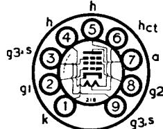
The BRIMAR 6870 is a Trustworthy high slope pentode for use as a small transmitting valve or as a video valve giving a larger output with low anode loads than an ordinary R.F. amplifying pentode.
