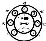
This miniature thermal delay switch has been designed to provide delay between the application of heater voltage and anode voltage in indirectly heated valves and mercury vapour rectifiers.
