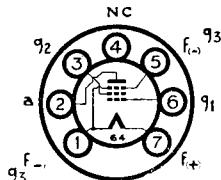
BRIMAR type 1T4 is one of the series of miniature battery valves introduced for portable radio equipment. It is suitable for the R.F. or I.F. stages of receivers employing A.V.C. Type 1T4 is well screened internally and will function satisfactorily as a high gain amplifier in deaf aid or other audio apparatus.
