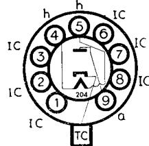
The BRIMAR PY81/17Z3 is an indirectly heated booster diode designed for operation in A.C./D.C. television receivers. The high working peak heater to cathode potential renders the use of a separate, highly insulated heater winding unnecessary.
