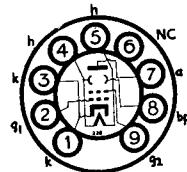
The 5A/170K is an indirectly-heated beam tetrode developed for general-purpose wide-band applications. It has a high mutual conductance, and a high ratio of mutual conductance to capacitance.
