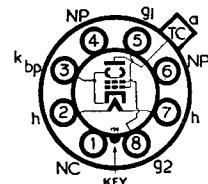
BRIMAR type 19BG6G is designed for use in the output stages of line time base generators in A.C./D.C. type Television receivers. The valve may be used in conjunction with BRIMAR type R12 rectifier to provide E.H.T. from line fly-back pulses.
