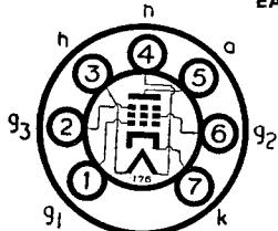
The BRIMAR type 6AK6 is a miniature output pentode with low heater consumption suitable for use in both AC and AC/DC equipment. It is particularly suitable where power economy and small physical size are of prime importance.
