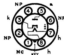
The BRIMAR type 6U4GT is an indirectly heated half-wave rectifier designed for efficiency diode service in television receivers. The high working peak heater to cathode potential renders a separate highly insulated heater supply unnecessary when a line output transformer of the "auto" type is used.
