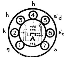
Heater Voltage ...    12.6 volts    Heater Current...    0.15 amps.
