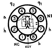
The BRIMAR type 35L6GT is an indirectly heated beam tetrode for use in the output stages of A.C./D.C. equipments where the operating voltages are low.
