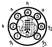
The BRIMAR 6BH6 is a medium slope, sharp cut-off R.F. Pentode designed for use in car radio and mobile equipment where economy of heater current is important.
