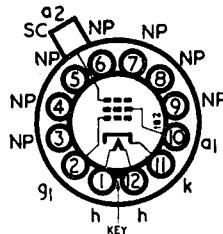
The C17HM/1 is a wide angle Teletube with a tetrode gun, ion trap, aluminized screen, and external conductive coating, for use in television picture monitors and similar applications. This tube is manufactured to a strict specification and is capable of providing high-grade pictures for television monitoring and industrial purposes.
