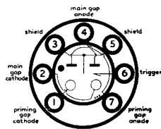
The G1/371K is a high-speed primed-trigger tube developed for use with the G10/241E Unidirectional Cold-Cathode Gas Filled Decade Counter for which a single cathode trigger tube is required as a coupling element between tubes. Its speed and general characteristics, however, make it a useful general component. It also has features which make it specially suitable for use in circuits where a high input impedance is required.
