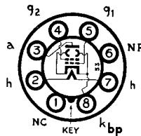
The BRIMAR type 6L6G is an indirectly heated beam power tetrode for use in the output stages of large audio equipment. Owing to the special construction only a small proportion of odd harmonics are produced and in push-pull connection large outputs may be obtained without distortion.
