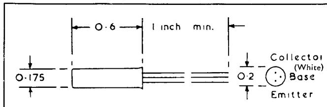
The TJ1, TJ2 and TJ3 are p.n.p germanium alloy junction transistors intended for use in audio frequency applications. The TS1, TS2 and TS3 have similar characteristics but are hermetically sealed and are smaller than the TJ1, TJ2 and TJ3.
