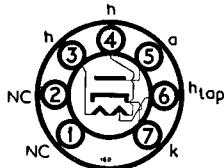
The BRIMAR type 35W4 is an indirectly heated half-wave rectifier for use in compact A.C./D.C. equipment.
