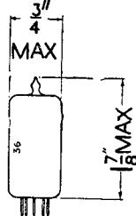
**Current Equipment Type****TYPE 6AU6****HIGH SLOPE****R.F. PENTODE**
