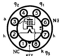
The BRIMAR type 6AG6G is an indirectly heated output pentode of high sensitivity for use in the output stage of radio receivers.
