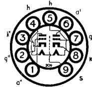
BRIMAR type ECC85 is a Noval based double triode intended primarily as an R.F. amplifier and frequency changer in F.M. receivers.
