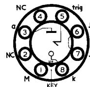
The G150/2D is a cold cathode, three-electrode, gas-filled triode. It has an activated cathode giving a low maintaining voltage, together with a good life performance.
