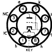
The 3A/167M is an indirectly heated triode of very high mutual conductance which has been developed for use in the output stages of wide band amplifiers, and for cascode low-noise amplifiers.
