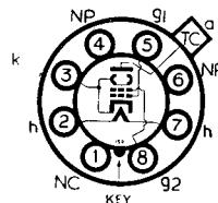
BRIMAR type 6BG6G is designed for use in the output stages of line time base generators in A.C. television receivers. The valve may be used in conjunction with BRIMAR type R12 rectifier to provide EHT from line fly-back pulses. For A.C./D.C. type television receivers the 19BG6G should be employed.
