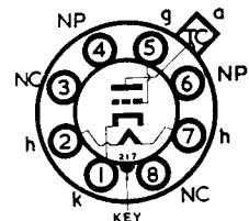
The Brimar type 6BD4 is a special triode for use as a shunt connected E.H.T. voltage regulator in television picture monitors, colour television receivers, etc.
