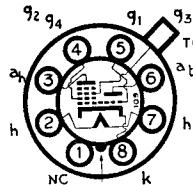
Note.—Type 6K8GT has Pin 1 connected to metal shell.
