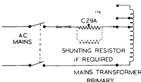
A Brimistor may be used to limit the switch-on surge in the primary of the mains transformer of T.V. and radio receivers. The use of a Brimistor will enable the rating of the fuse or other protective device in the primary circuit to be reduced, and so give more efficient protection from over-load due to component breakdown.
