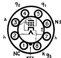
The BRIMAR type 25A6G is an indirectly heated power pentode for use in A.C./D.C. equipment where the operating voltages are low.
