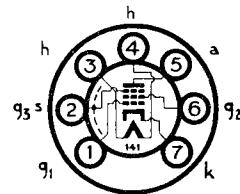
The BRIMAR 12AC6 is a vari-mu pentode for use in car radio receivers for operation direct from the 12-volt battery without the use of a vibrator H.T. system. It is designed to operate over the range of voltage variation normally encountered with car batteries.
