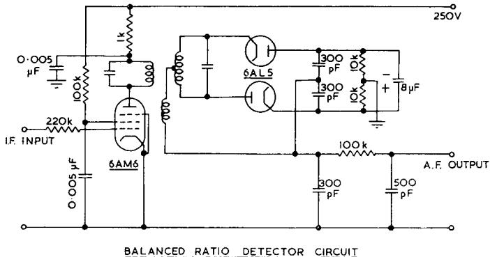
BALANCED RATIO DETECTOR CIRCUIT
