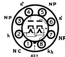
The BRIMAR type 5Z4G is an indirectly heated full-wave rectifier for A.C. mains operation.
