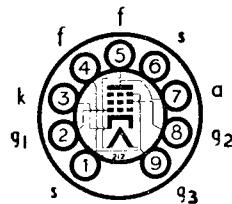
The Brimar EF89 is a high slope R.F. Pentode particularly suitable for use in F.M. receivers.
