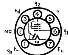
BRIMAR type 1S5 is one of the series of miniature battery valves introduced for portable radio equipment. It is designed for use as detector, A.V.C. and audio amplifier valve in superheterodyne receivers. Special care has been taken in the manufacture of type 1S5 to reduce noise and microphony to a low level.
