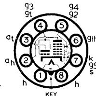
The BRIMAR type 7S7 is an indirectly heated triode-heptode of the "all glass" construction, fitted with a lock-in type base. Type 7S7 features high conversion, together with high anode impedance and will operate efficiently at frequencies up to 100 Mc/s.
