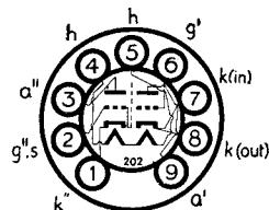
The BRIMAR PCC84/7AN7 consists of two separate high slope triode units designed for use in VHF cascode amplifiers. Normally, triode 1 is operated as a grounded cathode stage directly coupled to triode 2 which is connected as a grounded grid stage. This gives a low noise input amplifier for use in television receivers for Band III. The shield connected to the grid of triode 2 keeps coupling between the two units to a minimum.
