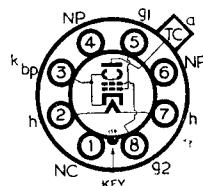
The BRIMAR 6CD6G is designed for television line time base output service in applications where the power requirements are greater than can be satisfied by the 6BG6G. Its features include high anode current at low anode voltage, and high ratio of anode to screen current. Type 6CD6G is suitable for scanning wide angle cathode ray tubes up to 21" in size. When used in conjunction with type 6U4GT, efficient operation may be secured at low H.T. rail voltages.
