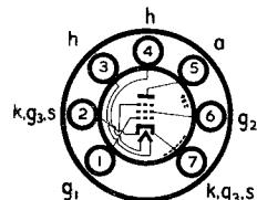
The BRIMAR type 6AK5 is a miniature R.F. Pentode intended for use as an R.F. or I.F. amplifier, particularly in wide-band applications. It is useful as an amplifier up to 400 Mc/s.
