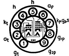
The BRIMAR PCL84 consists of a medium-high- $\mu$  triode and a high slope pentode in a miniature envelope on a noval base. The pentode section is intended for use as a video amplifier and will provide a larger current swing than high slope R.F. pentodes which have been used hitherto. The other section is a general purpose triode for use as a cathode follower, oscillator, etc.
