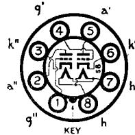
The BRIMAR type 6SL7GT is an indirectly heated valve comprising two high-mu triodes in one envelope. With the exception of the heaters, the connections to each assembly are brought out to separate base pins. Type 6SL7GT may be used as L.F. amplifier or phase inverter and in certain cases the two units may be connected in cascade to give a very high overall gain.
