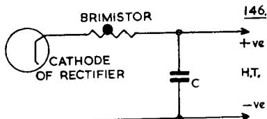
146. In order to reduce the switch-on current surge obtained with the large reservoir condensers associated with condenser input filters, a Brimistor should be connected between the rectifier cathode and the H.T. lead to the reservoir condenser and the H.T. leads as shown. The types to be used are as follows:
