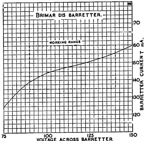
BRIMAR type D15 is a barretter suitable for use with the 0.15 amp. series of valves.
