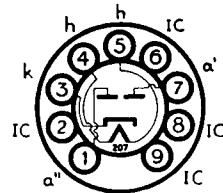
The BRIMAR EZ81 is a miniature noval-based full wave rectifier for use in radio receivers and amplifiers using a common heater supply.
