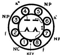
The BRIMAR type 5Y3GT is a directly heated full-wave rectifier for A.C. mains equipment of moderate power requirements.
