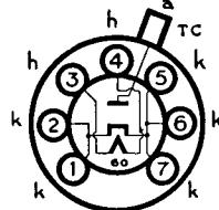
The BRIMAR type R10 is an indirectly heated half-wave rectifier of the "all glass" construction, fitted with a miniature type base. It is particularly suitable for use in portable oscilloscopes.
