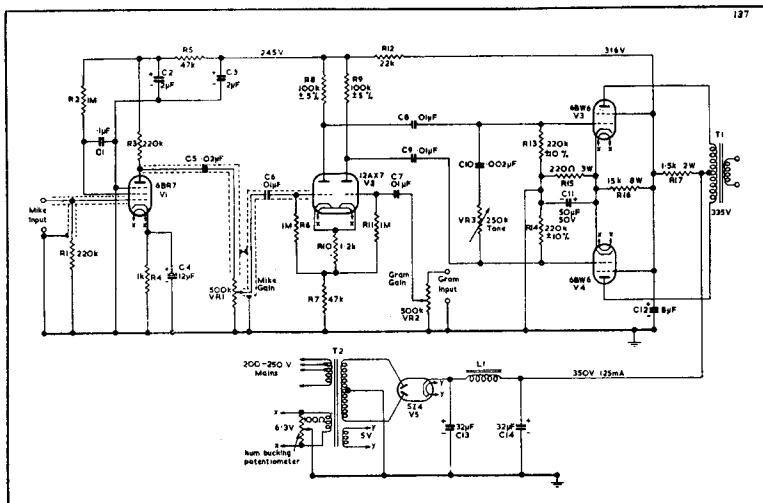
Output transformer impedance 10,000  $\Omega$  anode to anode.
