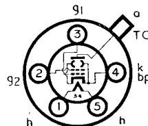
The BRIMAR type 807 is an indirectly heated beam tetrode for use in the output stages of large audio equipment. The valve is fitted with a low-loss base and may be used as R.F. amplifier or frequency multiplier in transmitters. Above 60 Mc/s the ratings must be reduced and at 120 Mc/s the ratings must not exceed 50 per cent. of the maximum.
