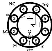
The G240/2D is a cold-cathode, three electrode, gas-filled triode. It has been developed for use in applications where a higher power is needed in the anode circuit than is obtainable with the G150/2D type.
