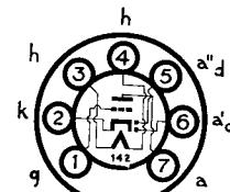
The BRIMAR 6AV6 is a miniature double diode triode for use in A.M. receivers for signal detection, A.G.C. and A.F. amplification.
