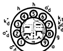
The type EABC80 is primarily intended for use as the demodulator/1st A.F. Amplifier in A.M./F.M. Receivers, one diode having a separate cathode. Diodes 2 and 3 should be used for discriminator circuits, Diode 1 for A.M. demodulator and A.G.C. circuits.
