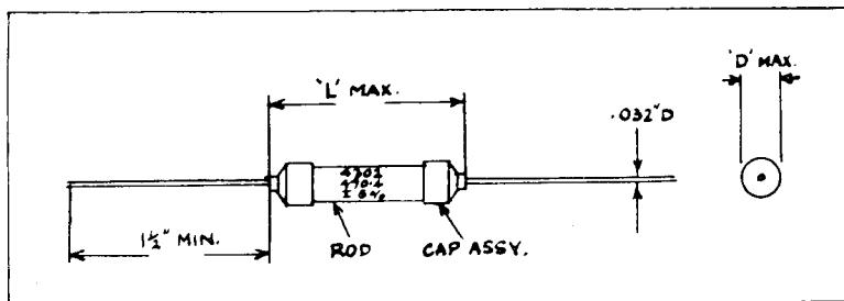
The resistance value is indicated directly by figures, followed by the symbol "U" for ohms, "K" for kilohms, or "M" for megohms.
