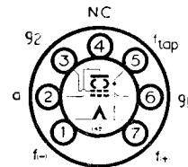
BRIMAR type 3V4 is an output valve for use in battery and A.C./D.C. Battery receivers where the H.T. supply is 90 volts. Compared with type 3S4 it features increased power sensitivity and reduced harmonic distortion.
