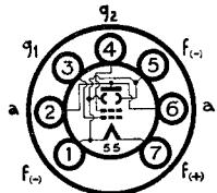
BRIMAR type 1S4 is one of the range of miniature battery valves introduced for replacement use in existing "personal" receivers. It has now been superseded by type 3S4.
