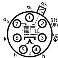
Heater Voltage ... ... ... 13.0 volts Heater Current ... ... ... 0.15 amp.
