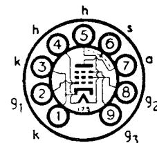
The BRIMAR 9D7 is a high slope R.F. pentode with a vari-mu characteristic for use in the I.F. stages of television and F.M. receivers using automatic gain control. It is suitable for use with both A.C. and A.C./D.C. operated receivers.
