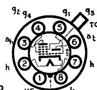
Note.—Pin 1 connected to metal shell.
