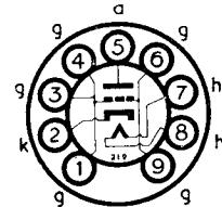
The BRIMAR 6AM4 is a miniature B9A based triode suitable for grounded grid amplifier or mixer use in the frequency range 470 to 890 Mc/s.
