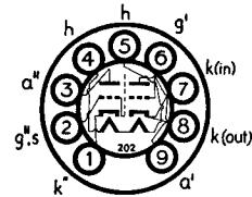
The BRIMAR ECC84 consists of two separate high slope triode units designed for use in VHF cascode amplifiers. Normally, triode 1 is operated as a grounded cathode stage directly coupled to triode 2 which is connected as a grounded grid stage. This gives a low noise input amplifier for use in television receivers for Band III. The shield connected to the grid of triode 2 keeps coupling between the two units to a minimum.
