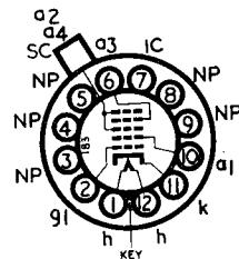
The Brimar C17SM is a rectangular 90° deflection angle teletube with electrostatic focus, an aluminized screen and external conductive coating. The screen colour is white with a grey glass faceplate with a transmission of approximately 70 per cent.
