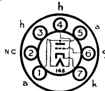
As oscillator or power amplifier, type 6C4 will operate efficiently at frequencies up to 150 Mc/s.
