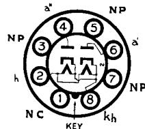
The BRIMAR type 5V4G is an indirectly heated full-wave rectifier for operation from A.C. mains. It will provide rather more output current than type 5Z4G and has a lower internal impedance.
