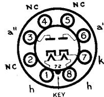
The BRIMAR type 7Z4 is an indirectly heated full-wave rectifier for use in A.C. and car radio equipment.
