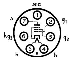
Heater Voltage ... ... 13.0 volts      Heater Current ... ... 0.315 amp.
