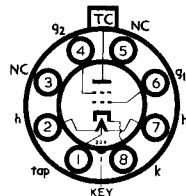
The SV-3D21A has been developed primarily for use as a blocking oscillator and pulse modulator. It is also suitable for use as a deflection amplifier, regulator or series valve in high voltage power supplies.
