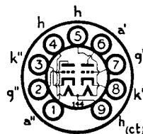
The BRIMAR type 12BH7 is a double triode with two independent low impedance units. It is designed particularly for television application, where one valve is suitable for use as frame oscillator and output stages for wide angle deflection cathode ray tubes.
