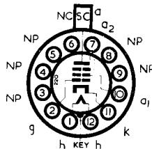
The BRIMAR C21NM is a rectangular 70° deflection angle Teletube with magnetic focus, a pentode gun incorporating an ion trap, aluminized screen and external conductive coating. The screen colour is white, with a grey glass faceplate with a transmission of approximately 67 per cent.
