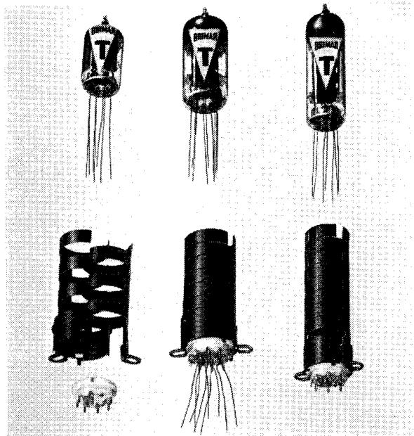
The use of close fitting blackened metal cans, improves cooling and disperses hot spots on the valve, and the resultant reduction in bulb temperature can improve life by four to five times.
