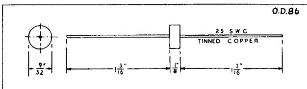
BRIMAR types M1 and M3 are miniature single plate selenium rectifiers which may be used to replace valve diodes in many applications, some advantages being the extremely small size, and absence of heater, simplifying the problem of avoiding hum.
