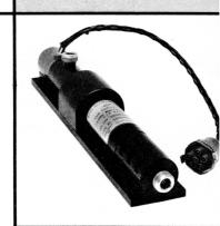
The EM-1016 features rugged ceramic and metal construction and focusing is provided by built-in periodic permanent magnets. These magnets are fully temperature compensated to allow operation from  $-55^{\circ}$ C to  $+85^{\circ}$ C. No additional cooling is required at these temperatures due to the integral heat sink/mounting flange supplied with the tube.
