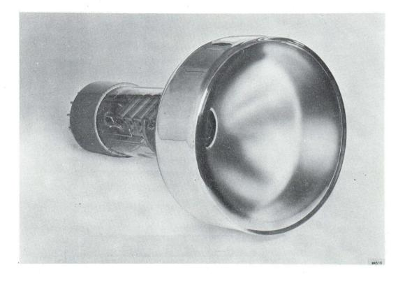
The 54AVP is an 11-stage photomultiplier tube provided with a caesium-antimony, semi-transparent flat cathode having a diameter of 111 mm. The highly sensitive uniform photocathode has a typical sensitivity of 60  $\mu$ A/lm and a spectral response lying mainly in the visible region, with its maximum at 4200 Å, as shown in the spectral response curve.
