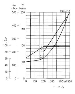
Closed cooling cycle with distilled water Overpressure = 1,5 bar  $t_1 = 60 \ ^{\circ}C$
