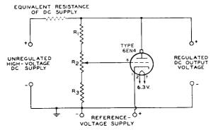
Typical performance data for this basic circuit with certain characteristics of the unregulated dc supply and related voltage-divider values are given in the tabulated data. Other combinations are feasible within the maximum ratings and the maximum circuit values for the 6EN4.
