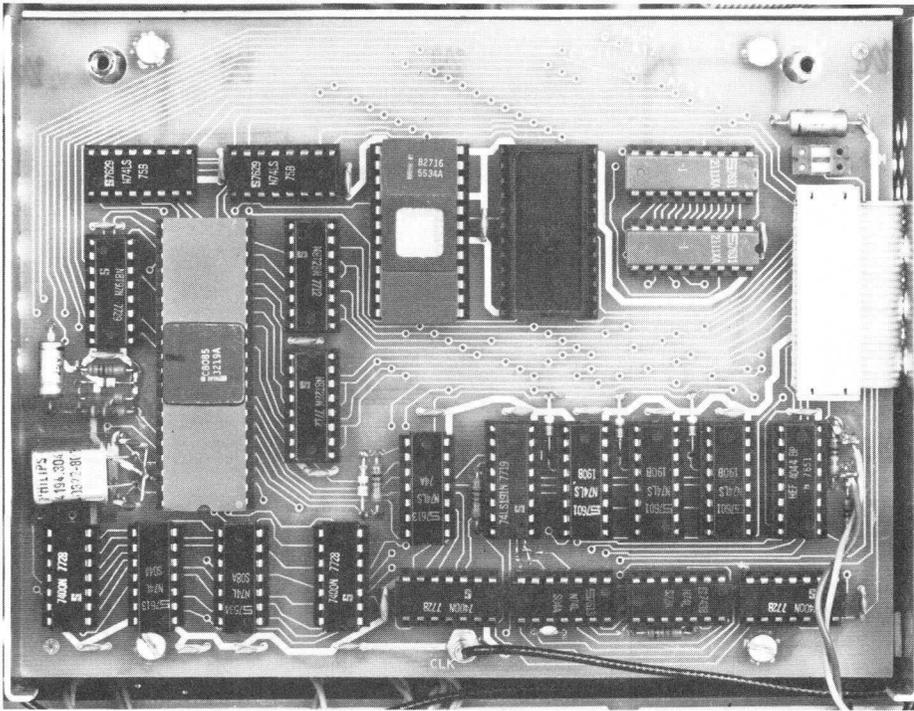
Fig. 3. The microprocessor is pcb-mounted with various associated components. Besides generally organizing all the delay features, it formats the display which warns the operator when the instrument is out of calibration or incorrectly set up.
