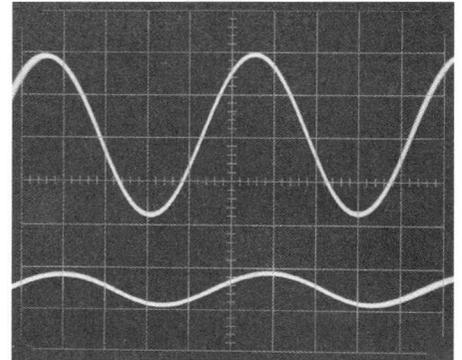
Fig. 3. At the output of the decoder crosstalk between the Left and Right channel is made visible using a dual beam oscilloscope. Displayed are: upper beam; right channel signal, lower beam; crosstalk on left channel.
