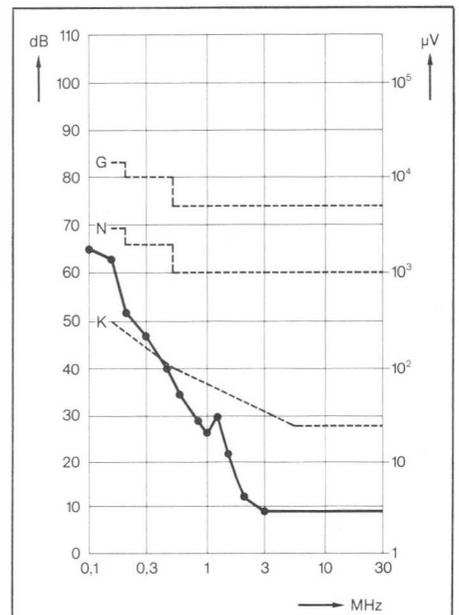
Fig. 1. Graph illustrates how for the great majority of the frequency spectrum the unit meets VDE 0875, curve K for mains interference, even through it is conservatively specified as meeting curve N.
