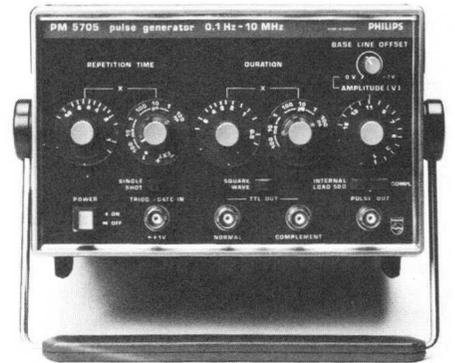
PM 5705 Universal pulse generator, frequency range 0.1Hz...10MHz features TTL line driver outputs and a 1...15V output with base line offset.
