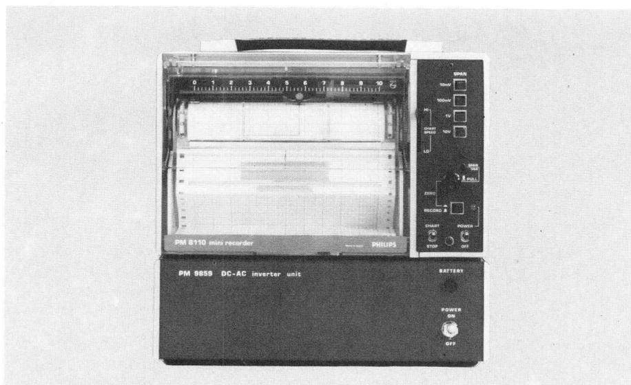
PM 8110 shown fitted with DC-AC inverter PM 9859
