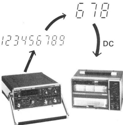
DAC gives high resolution analog recording in this case on Philips mini recorder PM 8110.
