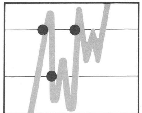
Fig. 1 is an enlarged detail of the RF waveform in fig. 2 and indicates how noise can cause the signal to pass through the trigger window and hence give a false count. This is eliminated in the PM 6650.
