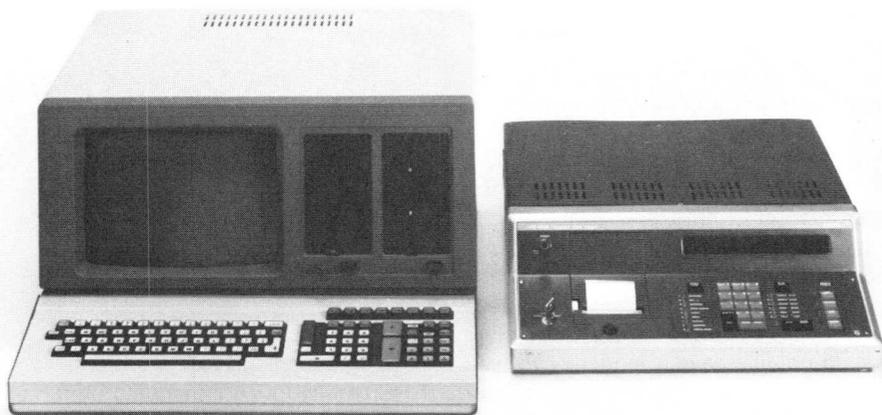
PM 4000 Data logger operating in conjunction with PM 4400 IEC-bus controller.
