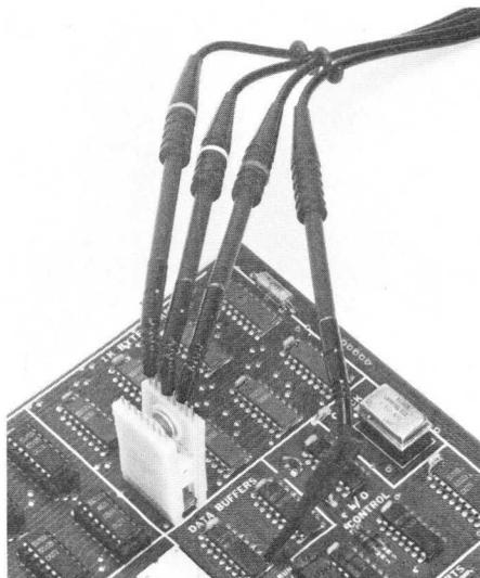
The colour-coded micro-miniature probes are supplied in touch, wire-wrap or hook styling. They can be used singly or in groups of four. Common earth connections may be used with up to nine probes.
