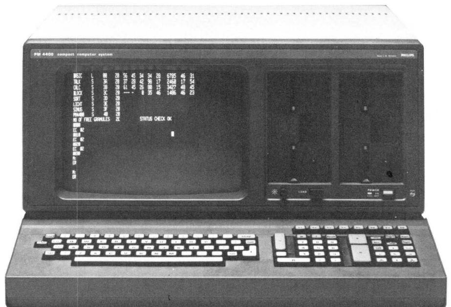
The PM 4400 IEC-bus controller is part of the family of products based on the PM 4400 compact computer system. The basic facilities of the PM 4400 are first described, followed by data and applications of the IEC-bus controller.
