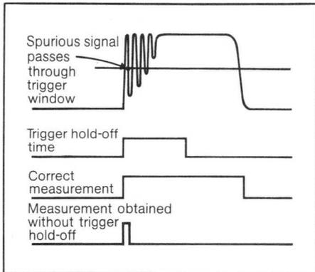
Fig. 2. The use of the PM 6622's variable trigger hold-off enables the influence of spurious signals such as ringing or relay bounce to be ignored and correct measurements obtained.
