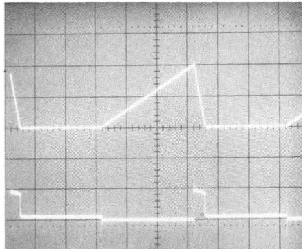
Fig. 1. Oscillogram of the power dissipation (lower trace) during the flyback period of the sawtooth voltage (upper trace).
