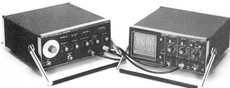
A typical educational application with PM 5131 being used in conjunction with oscilloscope PM 3226.
