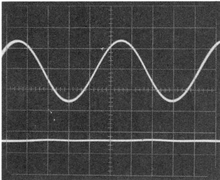
Fig. 4. After alignment, the crosstalk between the L and R channel has been minimized, as indicated by lower beam.
