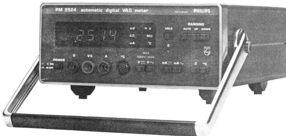
This autoranging digital meter measures voltage, current, resistance and temperature with high accuracy and reliability, plus excellent resolution with a  $4\frac{1}{2}$  digit display. The desired parameter is push-button selected and the autoranging facility ensures maximum resolution for every individual measurement. The correct symbol for the parameter being measured is automatically indicated. The red, 11mm high LED's are very easy to read.
