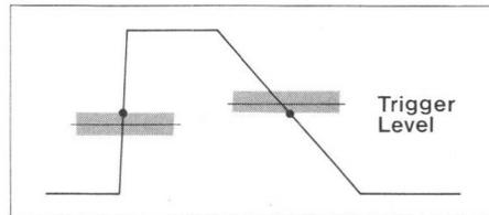
Fig. 3. Automatic hysteresis compensation shifts the hysteresis band on positive slopes downwards and on negative slopes upwards, with a value of half that hysteresis band.
