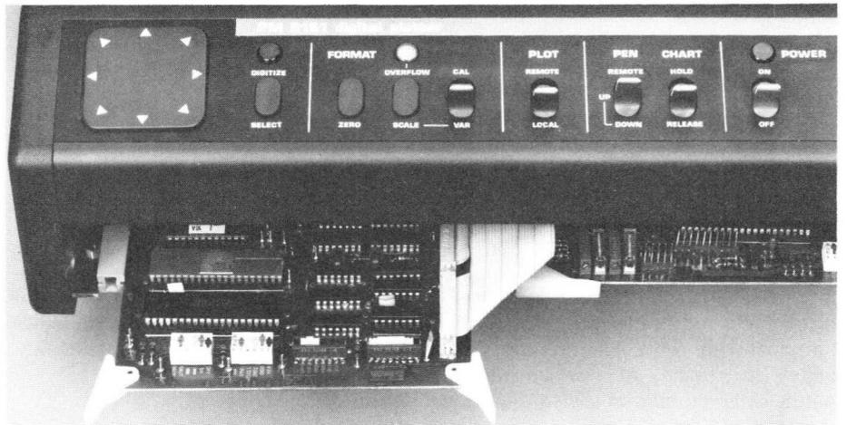
A detail showing the very simple control panel and the ease of access of the printed circuit boards.
