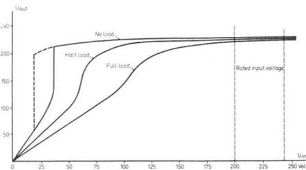
Fig. 2. Illustrates input/output voltage characteristics of model PE 1402.
