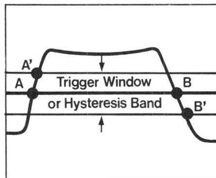
Fig. 3. Automatic hysteresis compensation ensures that triggering takes place at the level selected i.e. AB and not A'B'.
