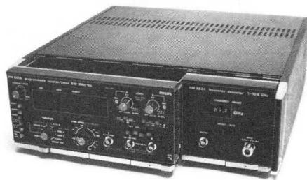
Fig. 5 illustrates the PM 6650 being used as a systems instrument in combination with sub-unit PM 6634.
