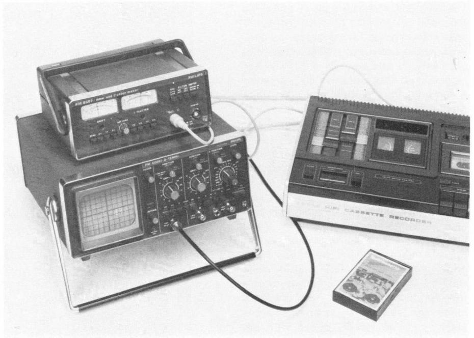
*PM 6307 being used to check a tapedeck for wow and flutter*
