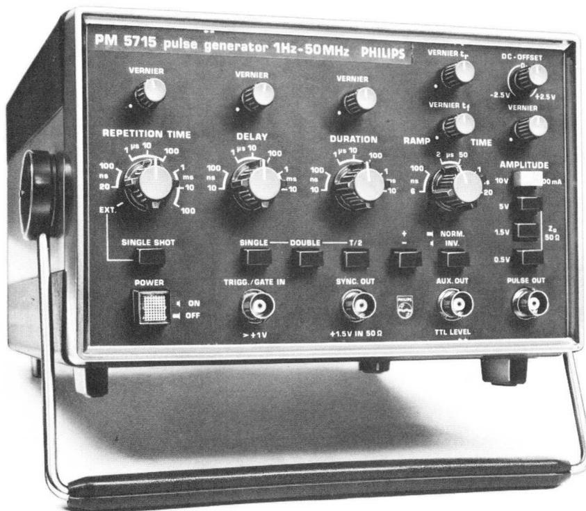
affect the auxiliary output. Coarse adjustment of the pulse rise and fall times (6ns to 500ms) is effected by means of a six-position switch. The rise and fall times have separate vernier controls for fine adjustment in each range. The 'output' pulses can be synchronously gated by an external signal. The first pulse coincides with the trailing edge of the gating signal, the last pulse is completed even if the gating signal ends during the pulse.
