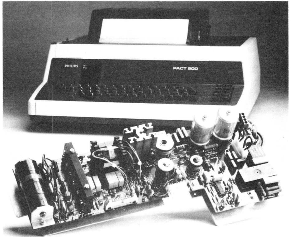
*This switched-mode power supply was designed for operation in a very restricted space. An important feature is the extremely high reliability requirement and high noise-suppression factor. It is for operation in the Philips Fact 200 telex machine.*
