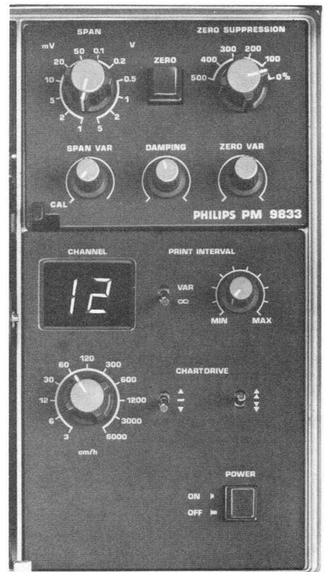
Fig. 4. Detail of range input module PM 9833, control panel and LED channel indicator.
