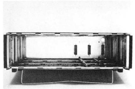
Fig. 6 demonstrates the convenience of the flush-fitting rear interconnection panel that powers and programs the sub-units.
