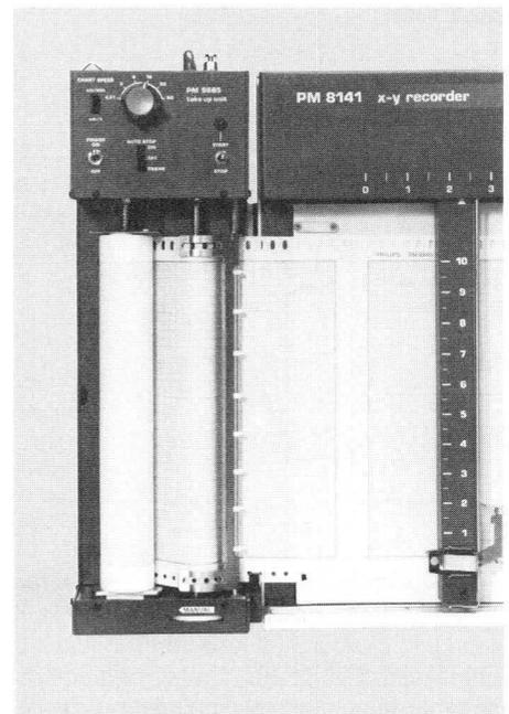
Chart transport unit PM 9885 shown fitted to X-Y recorder PM 8141.
