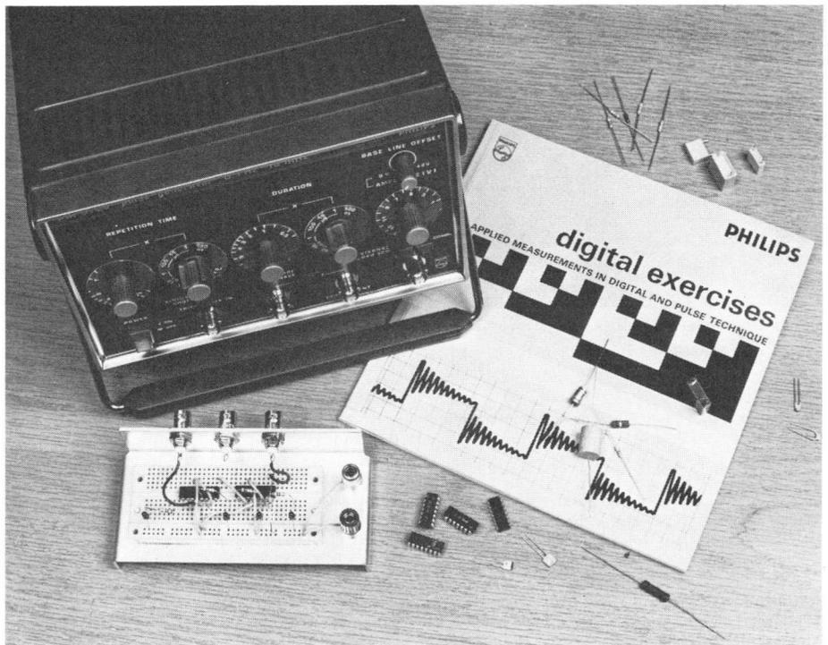
domain reflectometry and the influence of matched/mismatched cables. The measurements on integrated circuits start with TTL-logic in different applications then C-MOS logic is introduced and compared with TTL. Finally there are some specific C-MOS exercises.
