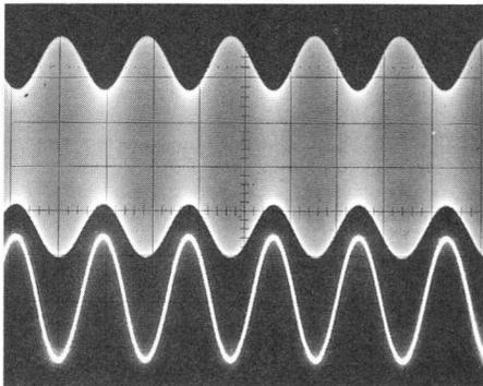
S curve with variable marker at 10.7MHz and fixed markers at regular intervals of 100kHz.
