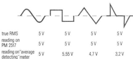
Fig. 1 shows comparison of reading accuracies between 'average' detecting and true RMS methods.
