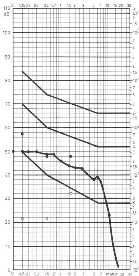
Mains interference level according to VDE 0875
