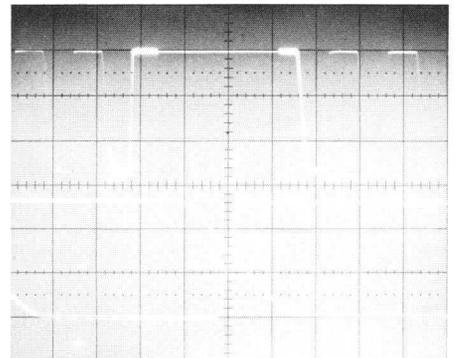
Fig. 2. Oscillogram showing the pulse-width measurement utilizing the increased accuracy achieved by using the alternate time base display facility.
