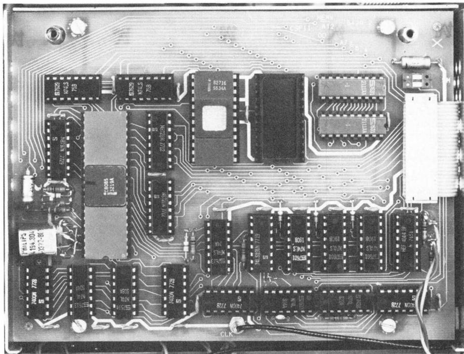
View of the microprocessor chip with its associated circuit components.
