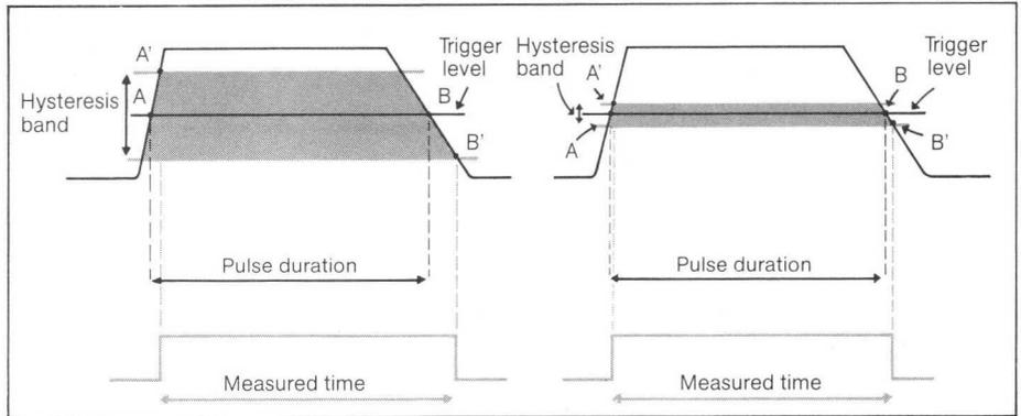
Fig.1. A wide hysteresis band (poor sensitivity) introduces measurement errors, as illustrated. In the PM 6620-series the low hysteresis voltage (typically 12mV<sub>p</sub>) minimises the error.
