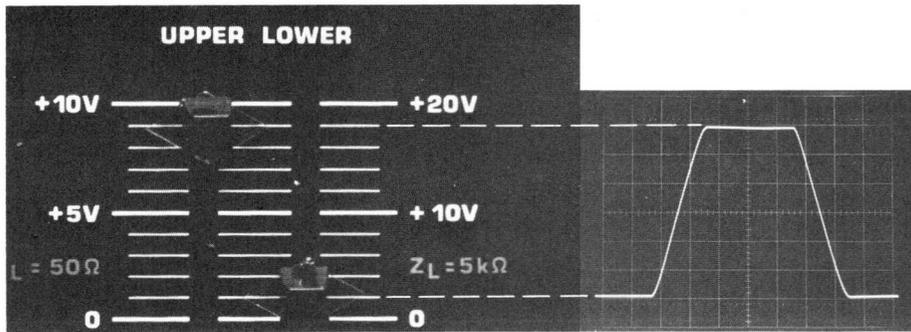
Fig. 1. Independent slide potentiometers for setting maximum and minimum pulse levels.
