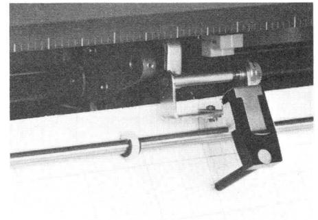
Fig. 3. Illustrates how the pen attachment can be clipped on so as to provide continuous recording of any one individual channel.
