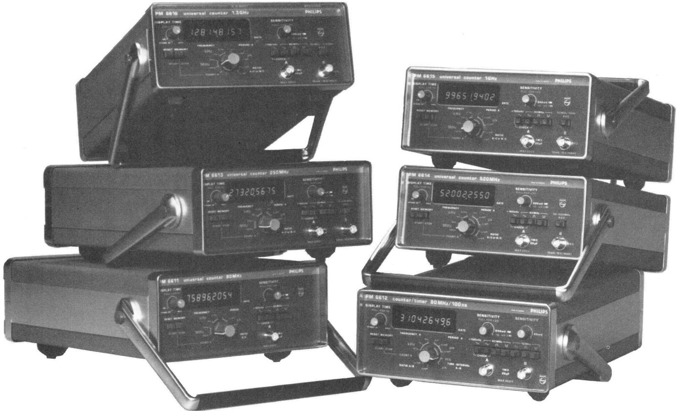
Wide frequency ranges from 10Hz up to 80MHz . . . 250MHz . . . 520MHz . . . 1GHz and 1.3GHz
