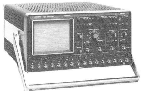
*The PM 3500 logic analyzer functions in both state and timing modes.*
