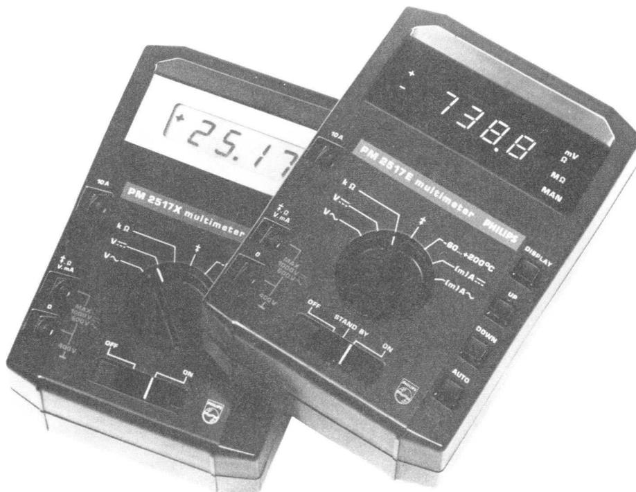
PM 2517 is a very compact general-purpose multimeter with an extremely high price performance ratio. It measures volts, current, resistance and temperature on a full 4-digit display (max reading 9999) with automatic ranging to ensure maximum resolution for every individual measurement.
