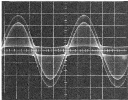
Fig. 2. To align for minimum crosstalk, the push-buttons for the R signal, a 1 or 5kHz tone and pilot are depressed. Shown is the resulting multiplex signal applied to the input of the decoder.
