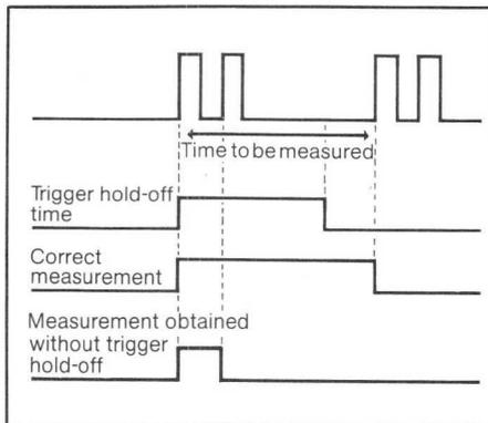
Fig. 3. Without trigger hold-off this double-pulse period measurement would be impossible.
