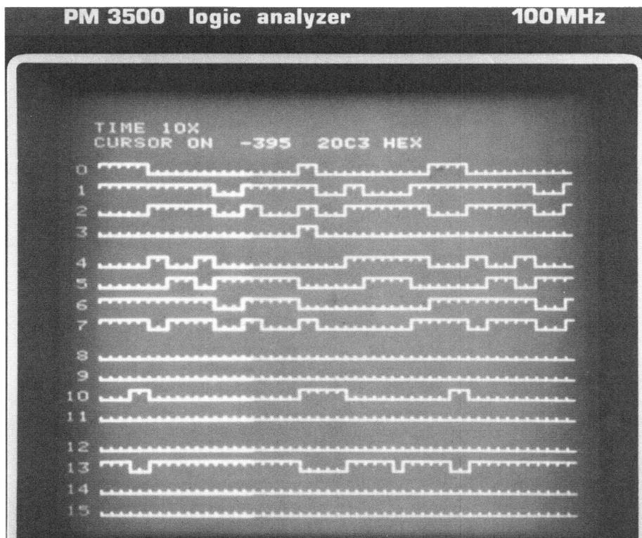
processors or minicomputers with multiple data lines often require even more. The PM 3500 and PM 3540 are optimized with 16 channels, this being adequate for general work. (For an operator to absorb more than 16 channels at one
