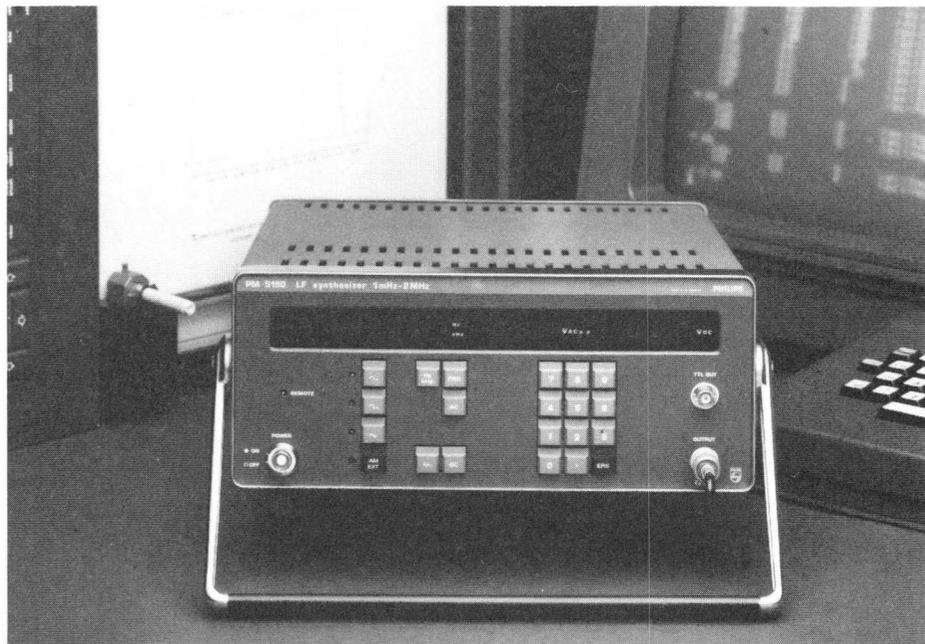
Automatic measuring and plotting of frequency response is made easier using the PM 5190.
