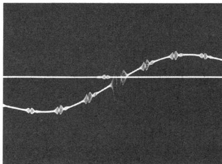
The luminance IF curve is aligned at its frequency of 38.9MHz.
