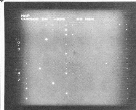
Use of a microprocessor in the PM 3500 analyzer allows simple switching between display formats for state analysis, providing binary, octal and hexadecimal tables with the added facility of a mapping mode.
