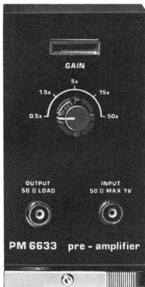
The PM 6633 is a low noise pre-amplifier that increases the input sensitivity of the main counter by a factor of 50. As illustrated, the sub-unit only occupies a space of 1/6th of the 19" rack and is therefore normally used in combination with the blank panel PM 9721N.
