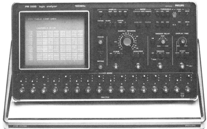
*The PM 3500 Logic analyzer which was introduced in 1979 is part of a new range of data test equipment which will be progressively extended*
