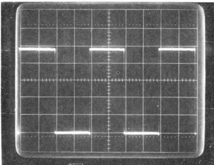
Fig. 1. Square wave at 5MHz
