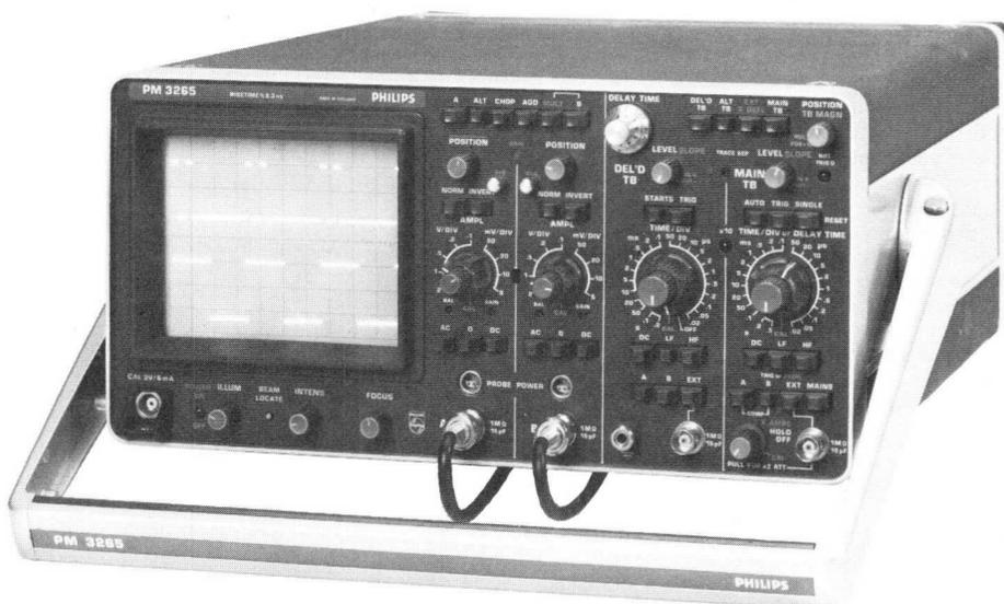
the delayed time base can be displayed simultaneously over the total screen width. It is therefore possible at all times, to see clearly which part of the pulse pattern is shown magnified.
