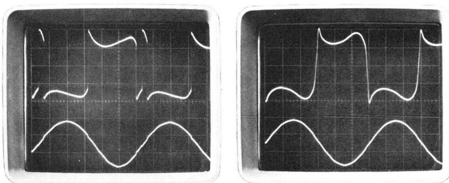
offered in alternative versions, therefore, whereby very high transient suppression is achieved with a slight loss in line stability. This is illustrated in figure 3. The suppression varies with the pulse widths and loads, but a typical improvement for a 11  $\mu$ s pulse is from an attenuation factor of 60 (-30dB) to over 110 (approx. -40dB) for only a slight loss in stability from 1 to 2% (for  $\pm 10\%$  mains variations).
