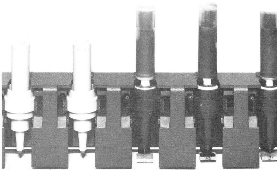
The pen capillary tubes are sealed off to prevent evaporation when not in use.
