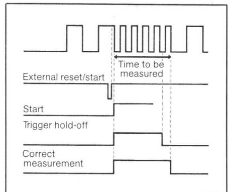
Fig. 4. The impressive combination of external reset/start and variable trigger hold-off enables this signal to be 'picked out' from the pulse train.
