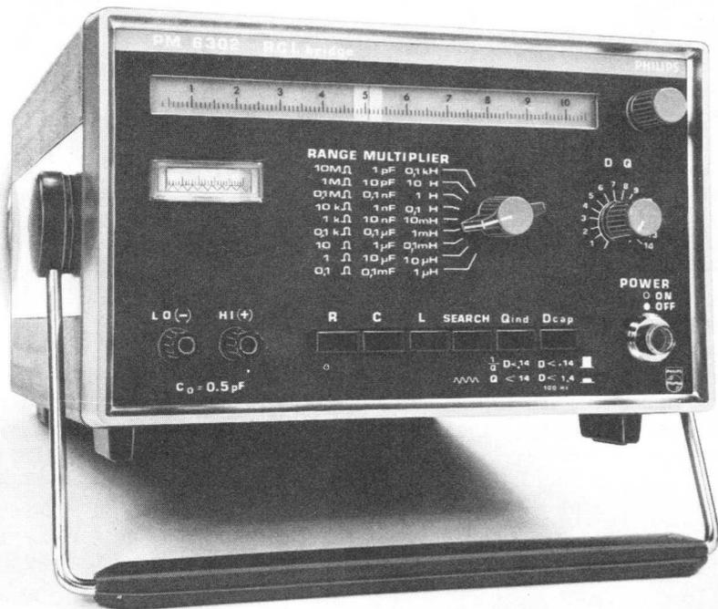
The PM 6302 is a modern transistorised RCL bridge with wide measuring ranges. Facilities for loss factor measurements, DC polarisation of electrolytic capacitors, connection of an external AC source (up to 20kHz) further extend the versatility of the instrument.
