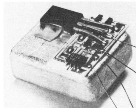
Low consumption crystal oscillator oven plus integrated temperature control.
