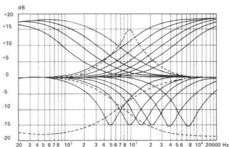
Fig. 2. Input channel equalizer curves.
