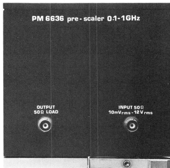
The PM 6636 extends the direct counting capability of the main counter to over 1GHz. This is achieved by pre-scaling (dividing) the input frequency. No tuning or level adjustment is required, because the input signal is automatically adjusted by a PIN diode attenuation circuit, as described for the PM 6610 series (page 152). At the same time this circuit performs the automatic noise attenuation function previously described on page 165.
