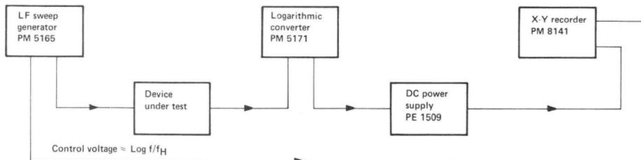
Fig. 1. Block diagram of measuring set-up.
