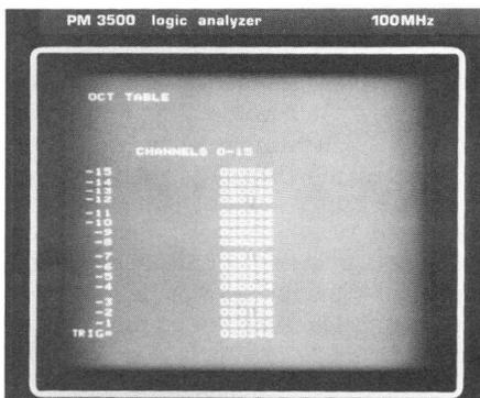
Octal and binary displays. At all times heading gives clear indication of display mode, cursor word and delay. The position of displayed words relative to the trigger word are given.
