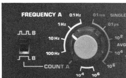
Conditioned pulse counting gives totaling of events on channel A. With the switch in the top position events are counted between a start and stop pulse. In the bottom position by a gate signal on channel B. Polarity and slope may be selected via the input controls.
