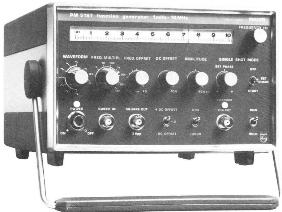
The PM 5167 function generator has a wide frequency range and extremely high output voltage (40V<sub>p-p</sub> open circuit). A wide variety of wave forms, excellent specifications, features like e.g. single shot mode with adjustable start, phase, sweep- and hold facilities and DC-offset and its compact construction make the PM 5167 a versatile tool for electronic laboratories, production groups and engineering design groups.
