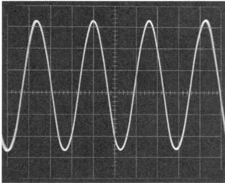
Fig. 1. Shows the 19kHz pilot tone from the PM 6456 applied to the input of the stereo decoder. Pilot tone and subcarrier frequency are checked and aligned.
