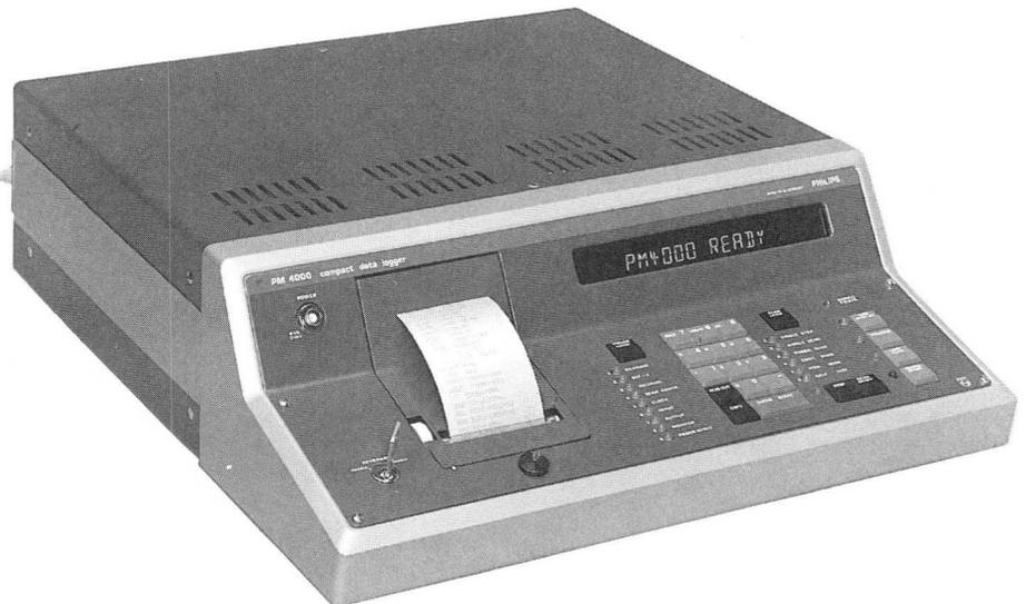
Thermocouple and Pt100 inputs are linearized by the logger and cold junctions of thermocouples can be connected to an isothermal input block. Where the thermocouple is a long distance from the datalogger, a compensation cable is used for the interconnection: up to four different external reference junctions allow four groups of cold junction temperatures to be programmed.
