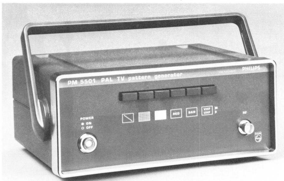
The PM 5501 colour pattern generator has been specially designed for black/white and colour TV alignment and service at the customer's house. The generator provides the 5 essential test patterns, necessary to make installations, fast checks and repairs on CTV and TV receivers possible. They are selected by push buttons.
