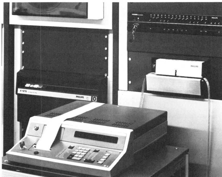
PM 4000 data logger operating in conjunction with a Philips P 800 series minicomputer.
