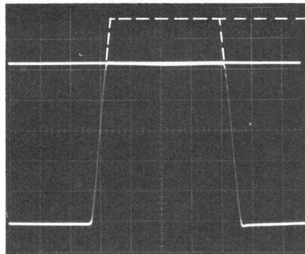
Fig. 2. Pulse limiter protects MOS circuit under test against excessive input pulse amplitudes.
