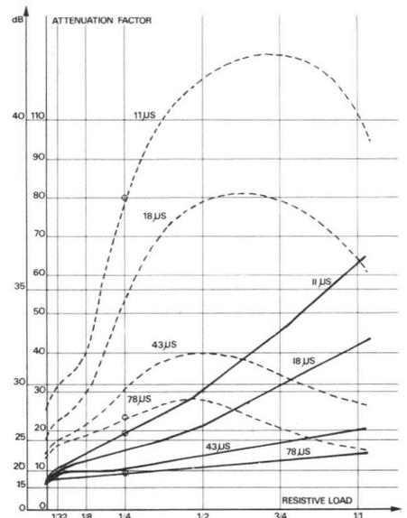
Fig. 3. Dotted lines show suppression with compensation winding disconnected, for transients having rise times from 11 to 78  $\mu$ s. Solid lines show suppression with winding connected. Thus for  $\frac{1}{4}$  load and on 11  $\mu$ s transient, the improvement is from an attenuation factor of approx. 20 to 80.
