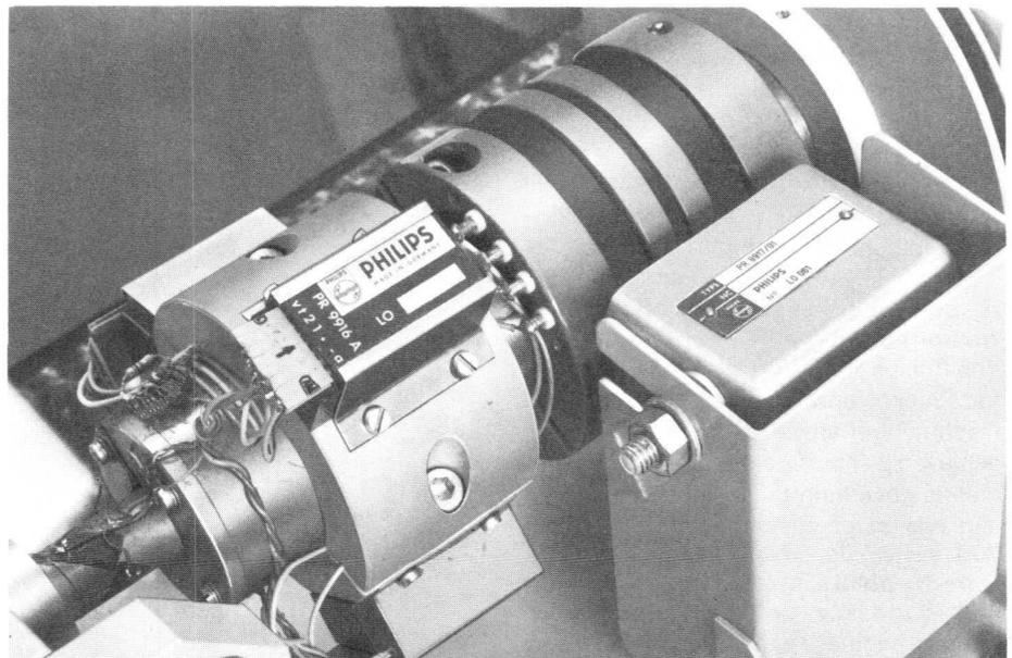
Torque measuring setup using the small size building blocks of the contactless transmission system for continuous operation.
