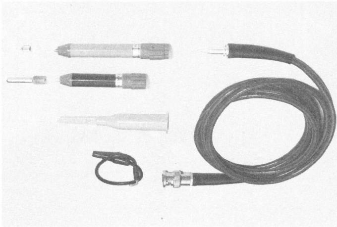
These probes are designed for use in the frequency range DC to 15MHz. The probe head is removable and can be selected to give an attenuation of either 1:1 or 10:1
