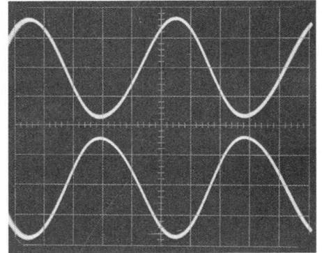
Fig. 6. Shows a full stereo decoded signal at the output of the decoder. Note: Both signals have equal amplitude and opposite phase. To obtain this display, the pilot, 1 or 5kHz and R=L push button are depressed.
