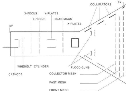
Fig. 4. Simplified diagram of the CRT design principles for the PM 3266, showing the set of meshes used in the high-speed transfer system and the scan magnifier lens system which produces the full scan display.
