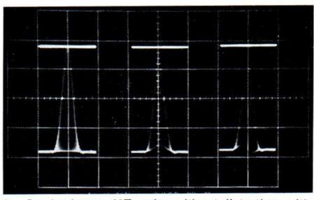
8. Carrier-borne 20T pulse without distortion, with pure amplitude distortion and pure group delay distortion (phase distortion)
