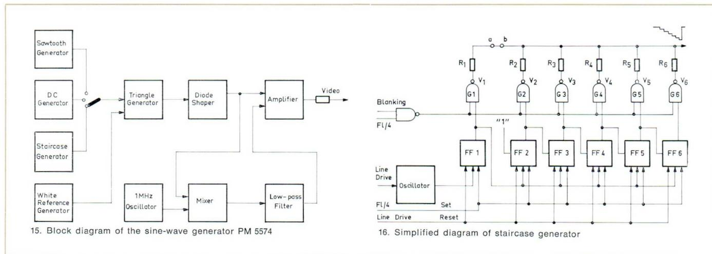
15. Block diagram of the sine-wave generator PM 5574
