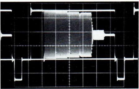
2. Multiburst with alternating white and black lines applied on sharp cut-off filter
