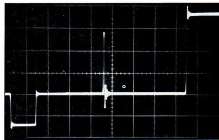
5. Pulse response of sharp cut-off filter to T pulse
