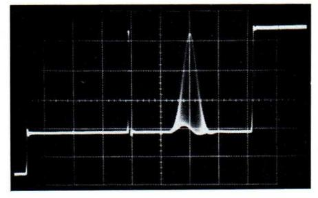
9. 2T, 20T carrier-borne pulse and bar after it has passed through the sharp cut-off filter
