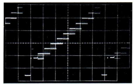
11. Staircase with superimposed subcarrier and burst
