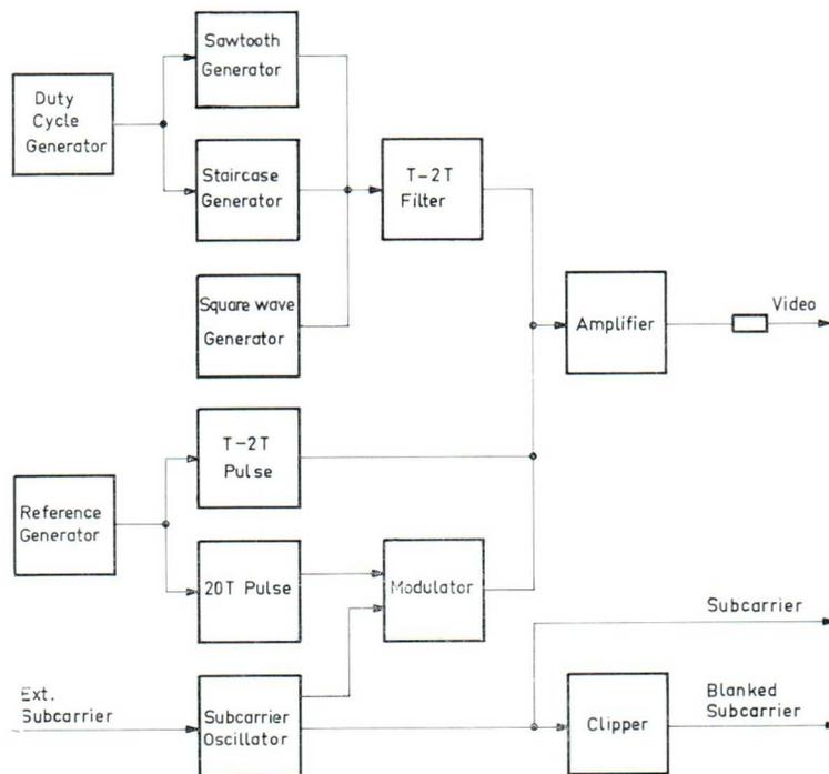
14. Block diagram of the pulse generator PM 5573
