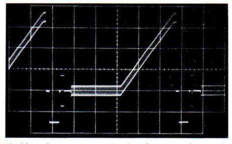
12. Line frequency sawtooth plus superimposed subcarrier with black duty
