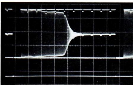
1. Sweep signal with marker and white ref. applied on sharp cut-off filter
