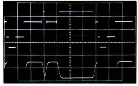
10. 20T pulse plus bar carrier-borne (chrominance) pulse after passage through non-linear network
