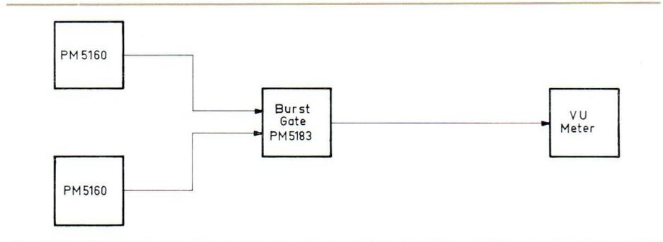
2. Block diagram for measurement of the response characteristics of a VU meter
