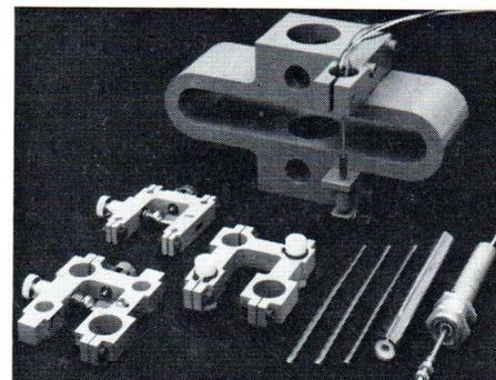
4. Extensometer in combination with a pull ring
