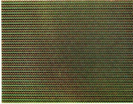
Venetian blinds due to incorrect phase of delay line circuit
