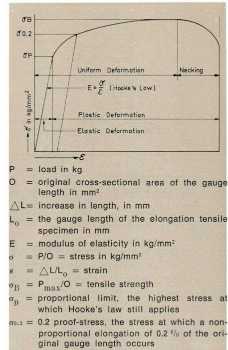
1. A typical stress-strain diagram
