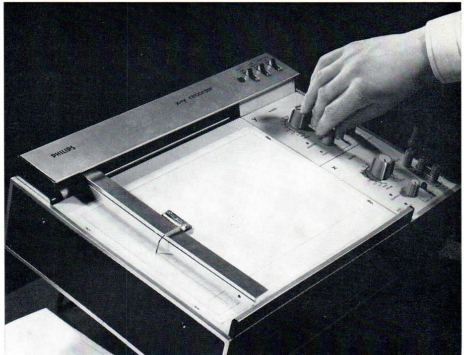
5. Flat bed X-Y recorder PM 8120; 0.05 mV/cm max. sensitivity; 0.25% accuracy
