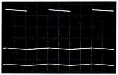
3. 50 Hz square wave displayed on oscilloscope. AC mode input is used to provide frame tilt
