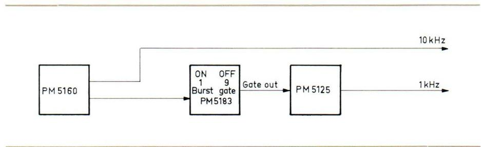
5. The PM 5183 can be used as a frequency divider. To obtain a sine wave, a PM 5125 can be synchronised with the gate pulse of the PM 5183
