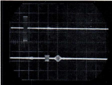
3. The various bursts involved in a reflection measurement displayed on a dual-trace oscilloscope. The reflected and cancellation bursts may be seen in the lower beam.
