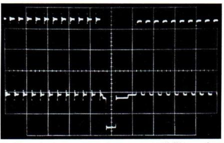
4. Transient response of sharp cut-off filter using 250 kHz square wave (rise times 90 and 180 nsec respectively)
