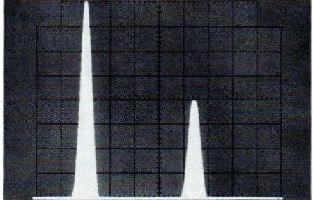
7. Spectrum of carrier-borne 20T pulse
