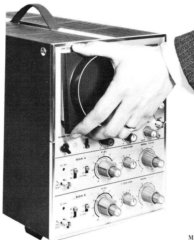
Fig. 8. Removing the protective cap and the measuring graticule
