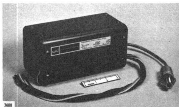
3088 circuit. All voltages are isolated from housing and RF output connector for maximum flexibility in circuit applications.
