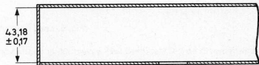
Fig. 4 Coupling section for YJ1500 into a waveguide R26 (used for measurements).
