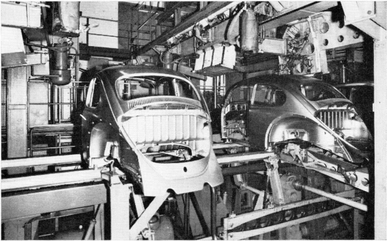
Fig. 4-27. Car production line showing partially assembled coachwork constructed by means of an ignitron-equipped welding system.
