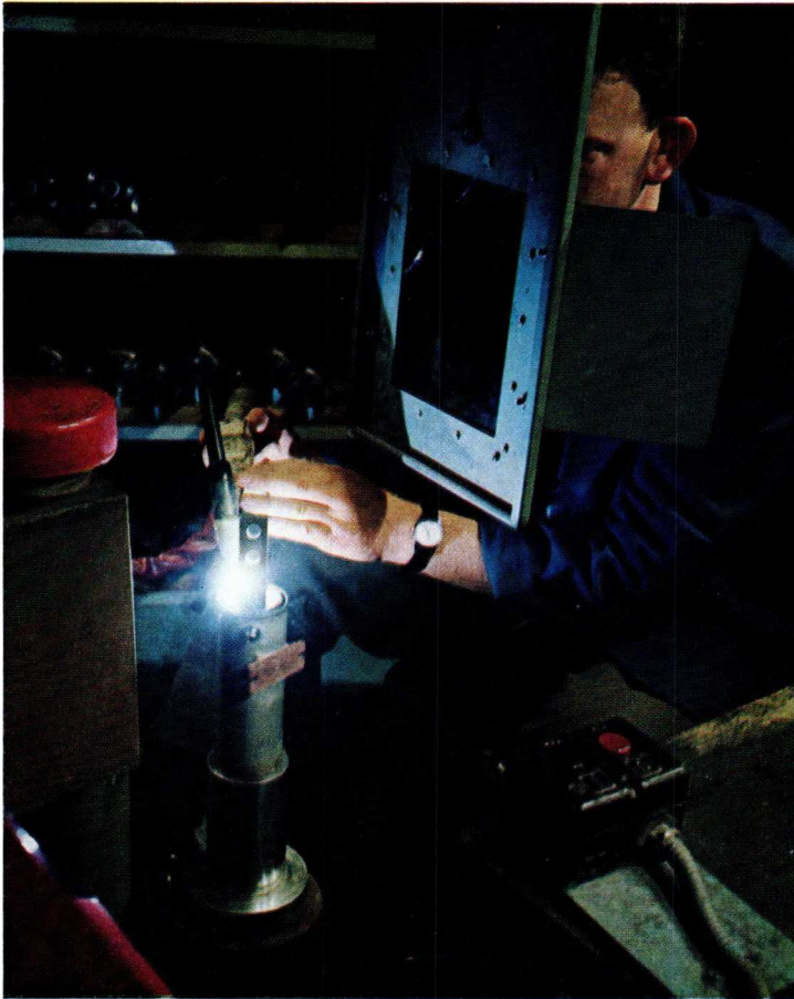
Fig. 4-5. The inner and outer walls of an ignitron water jacket being welded together during manufacture.
