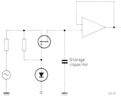
Fig.67 Sample and hold circuit.
