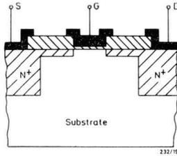
Fig.19 Cross-section through MOS-FET with one gate (see also Plate C).
