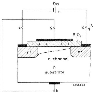
Fig.11 Schematic cross-section through a MOS field-effect transistor, n-channel depletion type (“normally-on”).
