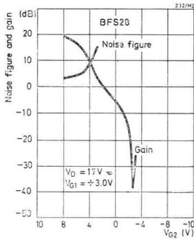
Fig.94 Noise figure and gain versus gate voltage for BFS28.
