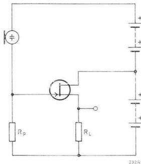
Fig. 45 Field-effect transistor in an impedance matching network for a capacitor microphone.
