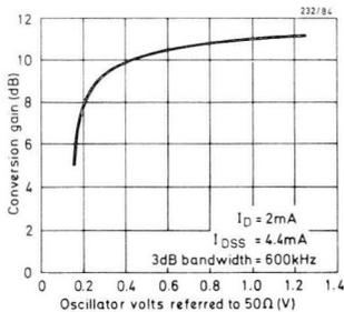
Fig.84 Conversion gain as a function of oscillator volts.
