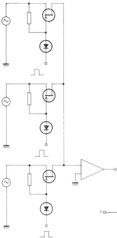
Fig.65 Analogue switches in data acquisition system.
