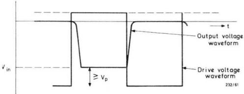
Fig.61 Switching waveform.
