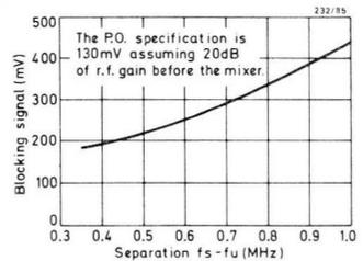
Fig.85 Blocking signal as a function of frequency separation.
