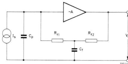
Fig.41 The pre-amplifier feedback loop shown partially decoupled.
