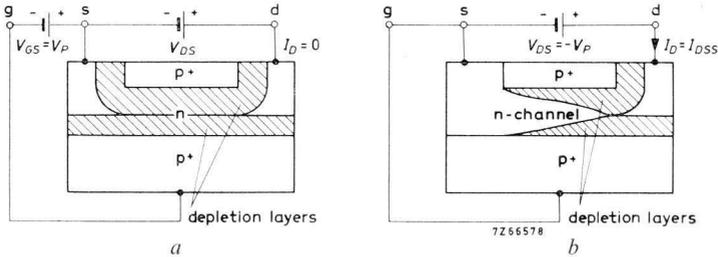
Fig.8 Pinch-off in the channel of a junction field-effect transistor. (a) by making  $V_{GS} = V_p$  at  $V_{DS} = 0$ ; (b) by making  $V_{DS} = -V_p$  at  $V_{GS} = 0$ . The upper and lower gate zones are connected as shown in Fig. 6.
