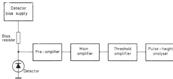
Fig.55 Block diagram of the electronics associated with solid-state detectors.
