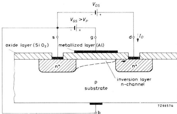
Fig.10 Schematic cross-section through a MOS field-effect transistor (MOS-FET), n-channel enhancement type ("normally-off").
