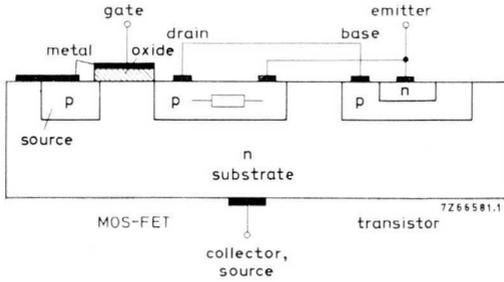
Fig.21 Schematic section through crystal of the integrated amplifier circuit TAA320 (See Plate E).
