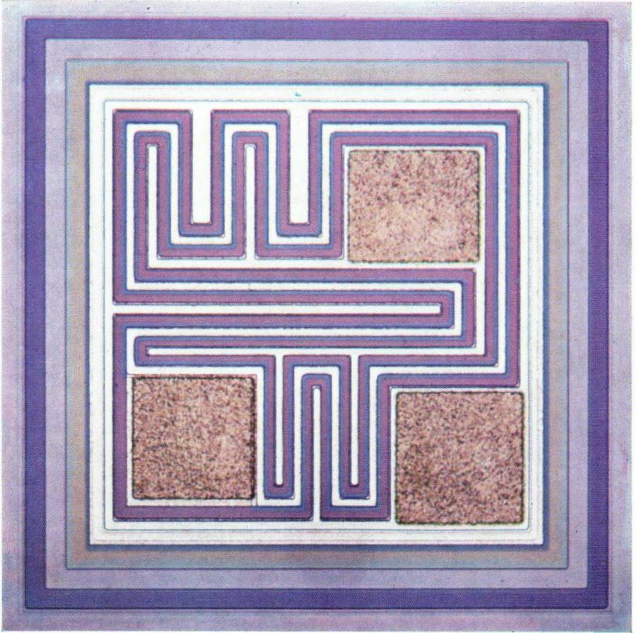
*Plate C. Closed structure (drain surrounded by gate) of a depletion MOS-FET (BSV81).*
