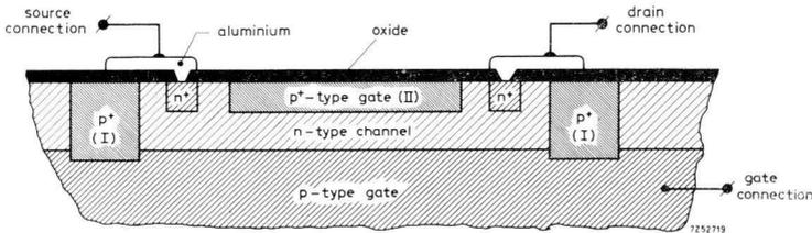
Fig.5 Structure of a junction field-effect transistor.
