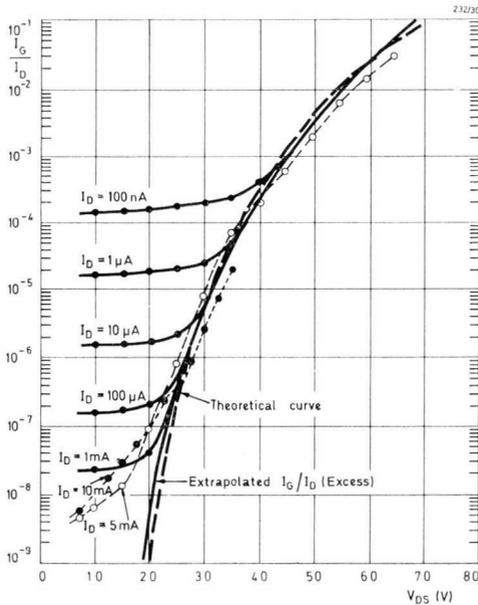
Fig.30  $I_G/I_D$  vs.  $V_{DS}$  with  $I_D$  as a parameter. Comparison of the excess gate current with the theoretical curve.
