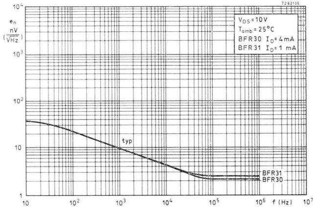
Fig.34 Equivalent noise voltage of a junction-FET as a function of frequency.
