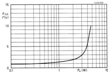
Fig.92 Distortion factor of the circuit of Fig. 91.
