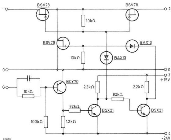
Fig.66 Bidirectional switch.
