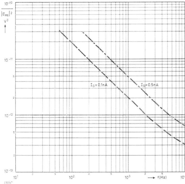
Fig.47 Graphical representation of the equations of  $\overline{|E_{eq}|^2}$  for two values of the gate current  $I_G$ .
