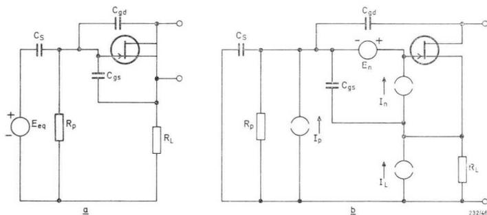
Fig.46 (a) Equivalent circuit of the network of Fig. 45. (b) Expanded equivalent circuit showing current and voltage sources responsible for the noise contribution of the network.
