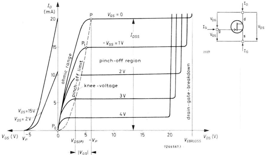
Fig.7 Characteristics of an n-channel junction field-effect transistor. Pinch-off voltage,  $V_P = -6$  V.
