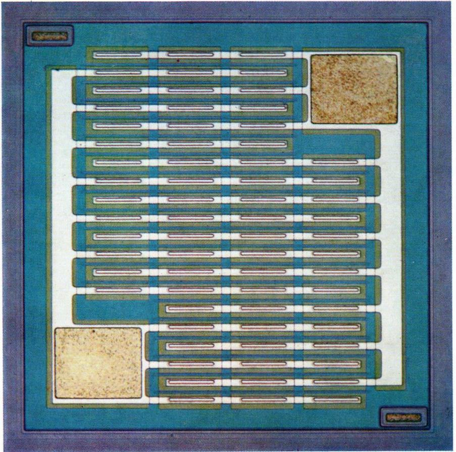
Plate B. Construction of an n-channel junction FET BSV78 to 80 in which  $W/L$  is about 5 times greater than in the FET of Plate A. This gives a very low on-resistance.
