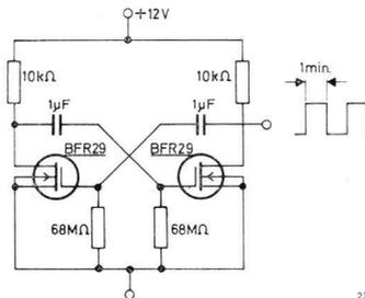
Fig.89 Multivibrator with long pulse duration.
