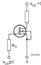
Fig.37 Simple circuit for adjustment of the operating point of junction and MOS field-effect transistors.
