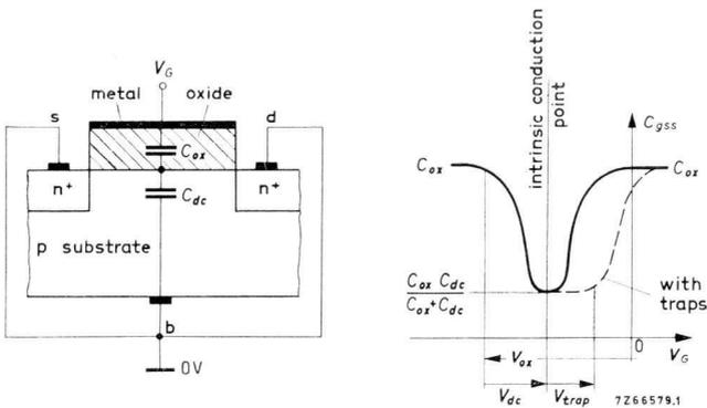
Fig.17 Dependence of the differential gate-source short-circuit capacitance  $C_{gss}$  (i.e. the capacitance for small signals) on the gate voltage for a normally-on n-channel MOS-FET.
