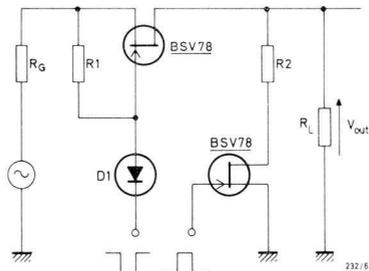
Fig.64 Series/shunt switch.
