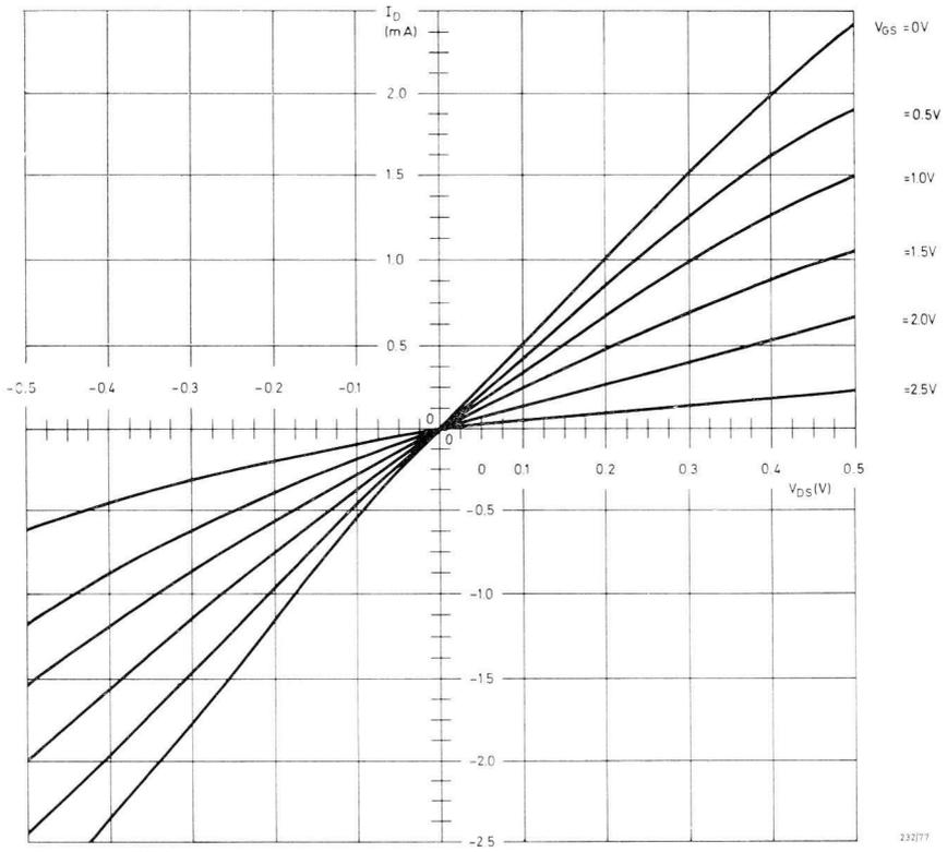
Fig.77 Characteristics of a FET as a symmetrical voltage-controlled resistor.
