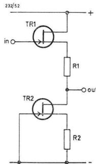
Fig.52 Simplified circuit diagram of the input stage.
