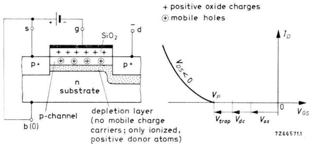
Fig.15 Elements of the pinch-off voltage  $V_p$  for a normally-off p-channel MOS-FET. A negative gate-source voltage is required for formation of the p-type inversion layer in the channel zone. The channel constriction at the drain end, caused by the drain current, is not shown here – drain current is assumed to be zero.
