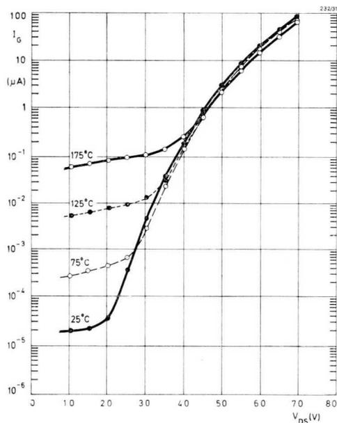
Fig.31  $I_G$  vs.  $V_{DS}$  with temperature as a parameter, measured at a constant drain current  $I_D = 1$  mA.
