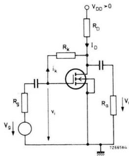
Fig.39 Stabilisation of the operating point of a normally-off MOS-FET by means of drain-gate feedback via  $R_D$  and  $R_K$ . ( $R_K$  reduces the input impedance).
