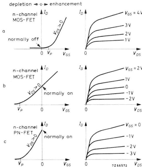
Fig.12 Examples of characteristics of field-effect transistors. (a) normally-off (enhancement type), (b) normally-on (depletion and enhancement type), (c) pure depletion-type (only found in junction FETs).
