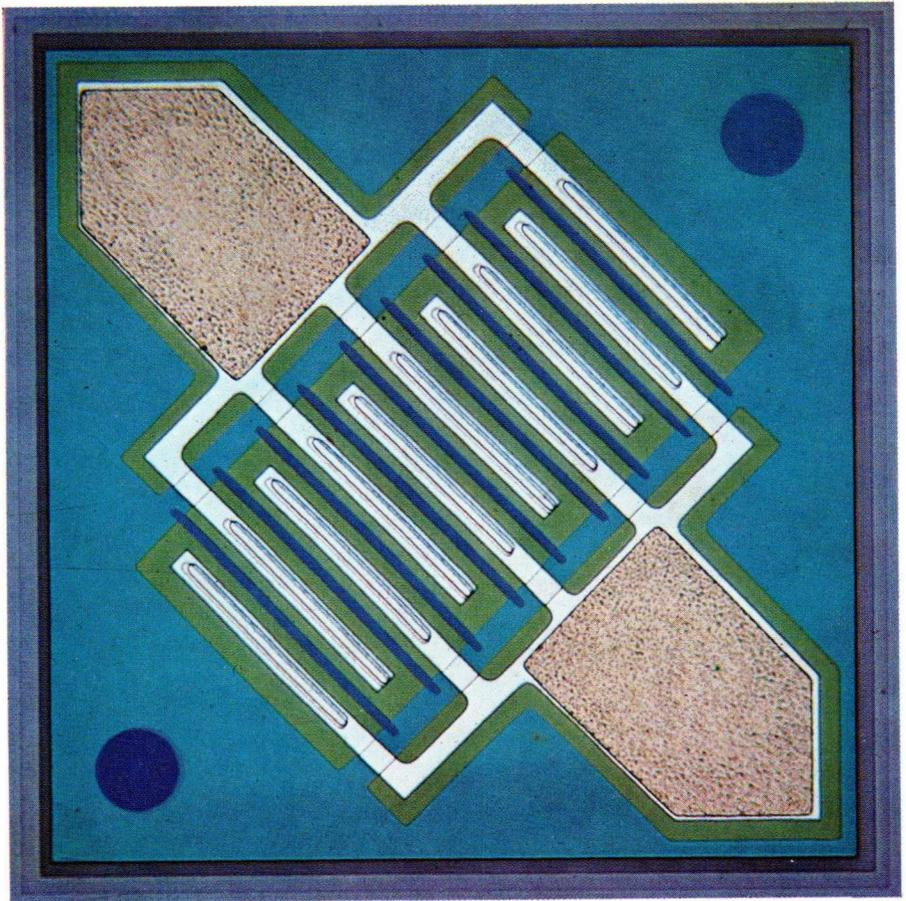
Plate A. Symmetrical construction of an n-channel junction FET (BFW10 . . . BFW13; see Fig. 9) yielding a low on-resistance and a low gate-capacitance.
