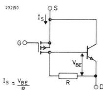
Fig.90 Electrical circuit of the TAA320.
