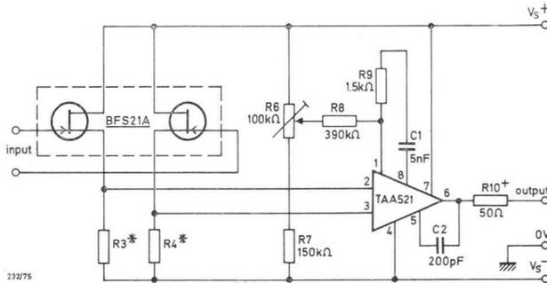
Fig. 75 Practical circuit for a FET pair used as a differential input stage for an operational amplifier. For  $V_S = \pm 9\text{ V}$ ,  $R_3 = R_4 = 47\text{ k}\Omega \pm 1\%$ . For  $V_S = \pm 15\text{ V}$ ,  $R_3 = R_4 = 82\text{ k}\Omega \pm 1\%$ .
