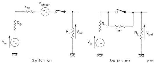
Fig.59 Elementary switching circuit.
