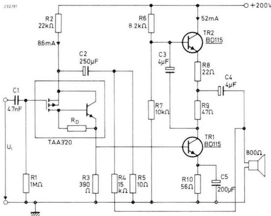
Fig.91 Circuit of a 4 W amplifier for a crystal pick-up input using the integrated circuit TAA320 and a transformerless push-pull class-A output stage.
