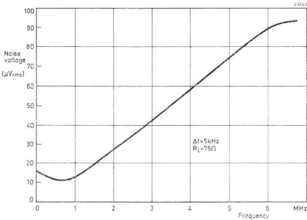
Fig.43 R.M.S. noise voltage at the output as a function of frequency.
