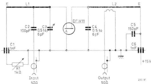
Fig.81 470 MHz common-gate amplifier.  $L_1 = 6$  cm of  $1/4$  in o/d Cu, tap at 4 cm from E;  $L_2 = 7$  cm of  $1/4$  in o/d Cu, tap at 4 cm from E. Characteristic impedance of line =  $70 \Omega$ .
