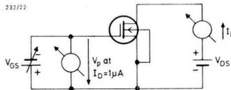
Fig.22 Measurement of the pinch-off voltage  $V_p$ . The value of  $1 \mu A$  given for  $I_D$  is an example only.  $V_p$  is often measured at lower drain currents.
