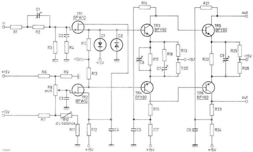
Fig.49 Three-stage vertical pre-amplifier for an oscilloscope with a pair of field-effect transistors in the signal input and the vertical shift control in the first stage.
