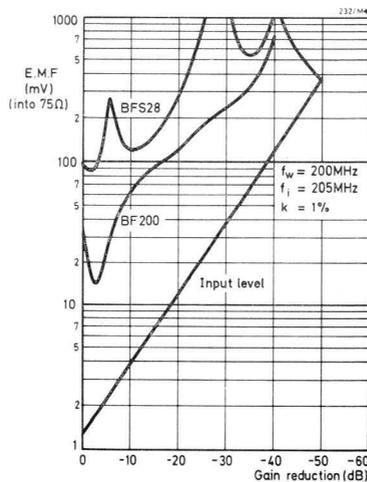
Fig.96 Interfering e.m.f. versus gain to give  $k = 1\%$  for BFS28 and BF200.
