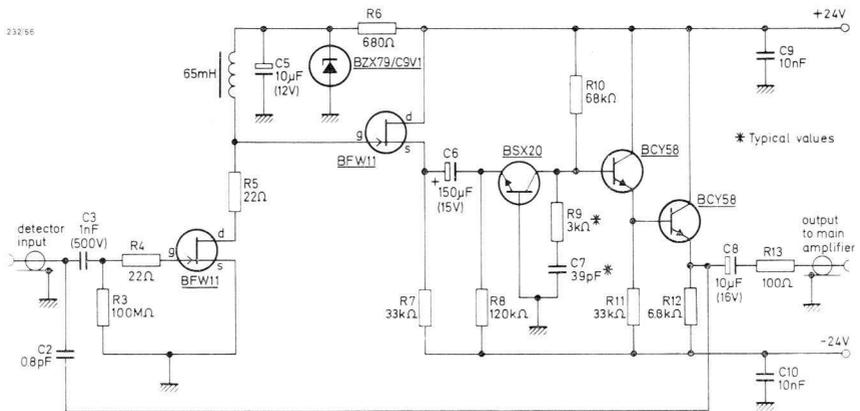
Fig.56 Pre-amplifier using field-effect transistors for silicon surface-barrier detector.
