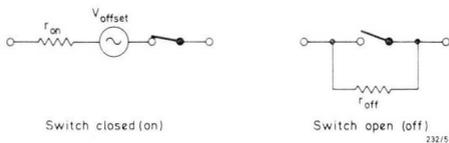
Fig.58 Errors generated by practical switch.
