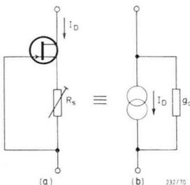
Fig.70 FET constant current source and its equivalent circuit diagram.
