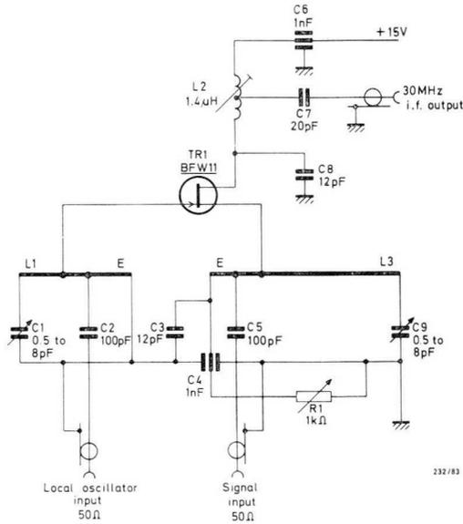
Fig.83 Mixer circuit.  $L_1 = 8.5$  cm of  $1/4$  in o/d Cu, gate tap at 2.6 cm from E, i.o. input at 1.5 cm from E;  $L_3 = 8.5$  cm of  $1/4$  in o/d Cu, signal input tap at 0.9 cm from E, source at 1.7 cm from E. Characteristic impedance of line =  $70 \Omega$ .
