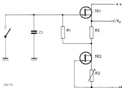
Fig.72 Linear sweep generator using FETs.
