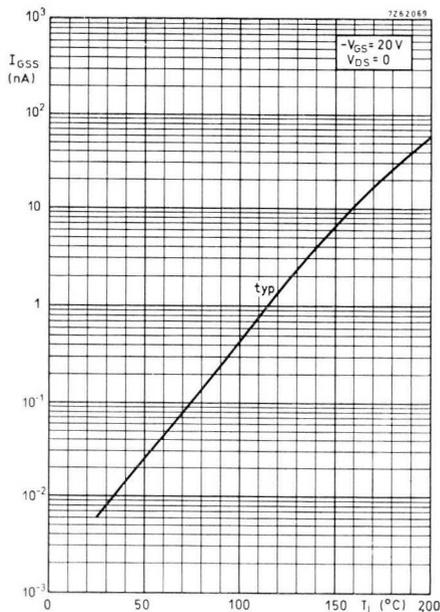
Fig.28  $I_{GSS}$  as a function of temperature for the junction FETs BFW10|11.
