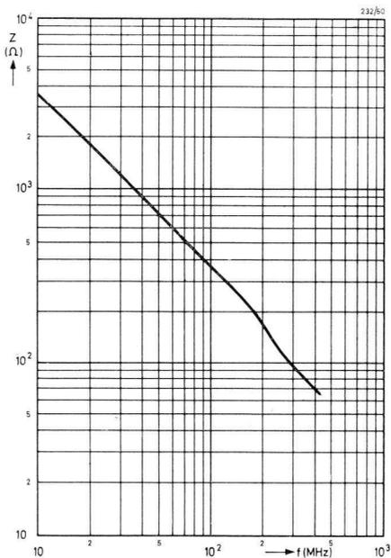
Fig.50 Input impedance of the pre-amplifier as a function of frequency.
