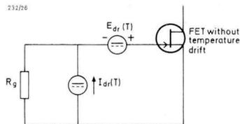
Fig.26 Temperature-dependent drift sources in a field-effect transistor.  $V_{dr}$  voltage drift;  $I_{dr}$  current drift;  $R_g$  resistance of signal source.
