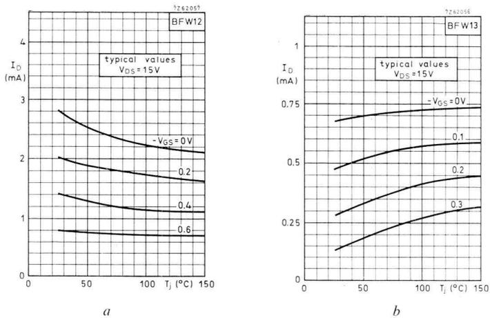
Fig.25 Temperature dependence of the drain current of two n-channel junction field-effect transistors. (a) In this case point Z in Fig. 24 is at a negative  $V_{GS}$  value, with predomination of temperature dependence of charge carrier mobility. (b) In this case point Z can be imagined as a positive  $V_{GS}$  value, with predomination of temperature dependence of  $V_p$ .
