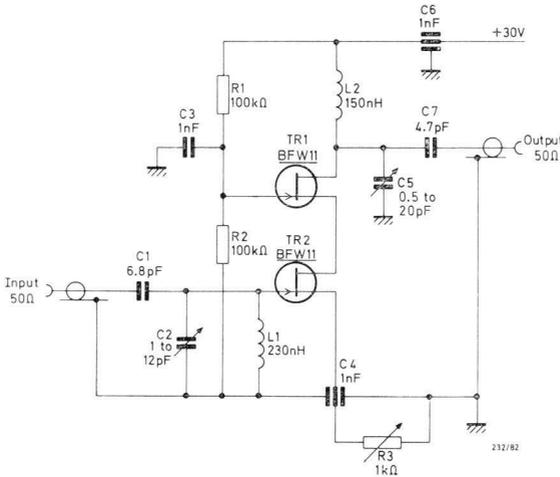
Fig.82 100 MHz cascode amplifier.
