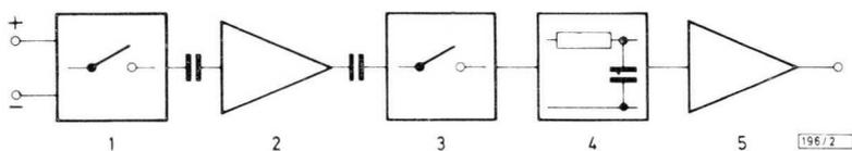
Fig.87 Block diagram of a chopper-stabilized amplifier.
