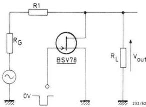
Fig.62 Shunt switch.
