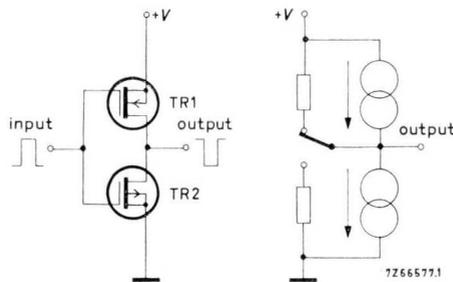
Fig. 4 Complementary inverter with MOS field-effect transistors. The leakage currents, represented as current generators in the equivalent circuit, are very small (of the order  $1\text{ pA}$  to  $1\text{ }\mu\text{A}$ ); the on-resistances are a few hundred ohms.
