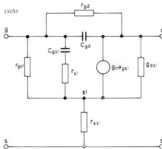
Fig.33 Small signal equivalent circuit for a FET.
