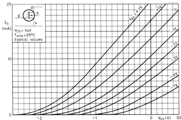
Fig.18 Influence of the source-substrate voltage  $V_{BS}$  on the control characteristic of a MOS field-effect transistor (*n*-channel MOS-FET BFR29 is used as an example).
