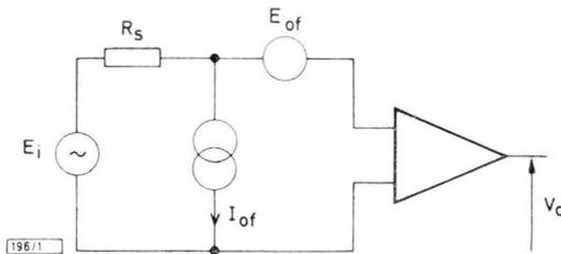
Fig.86 Equivalent circuit of the amplifier input.
