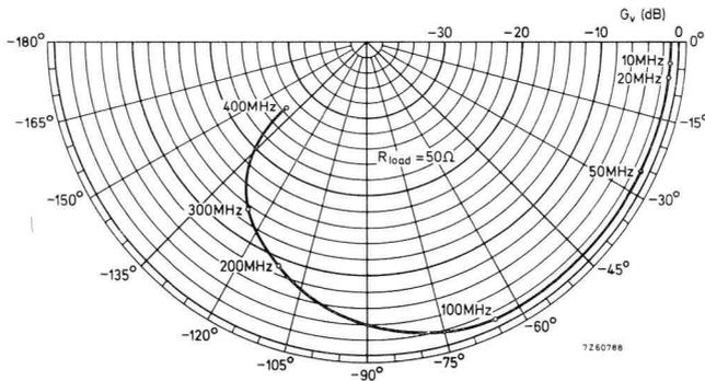
Fig.54 Polar diagram of the gain and phase angle versus frequency at a load impedance of  $50 \Omega$  for the circuit of Fig. 53a.
