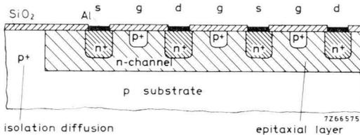
Fig.9 Cross-section through the crystal of the n-channel junction field-effect transistor BFW10, at right angles to the "teeth of the comb" of Plate A.
