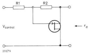
Fig.79 Linearization of  $r_{ds}$  by means of feedback.
