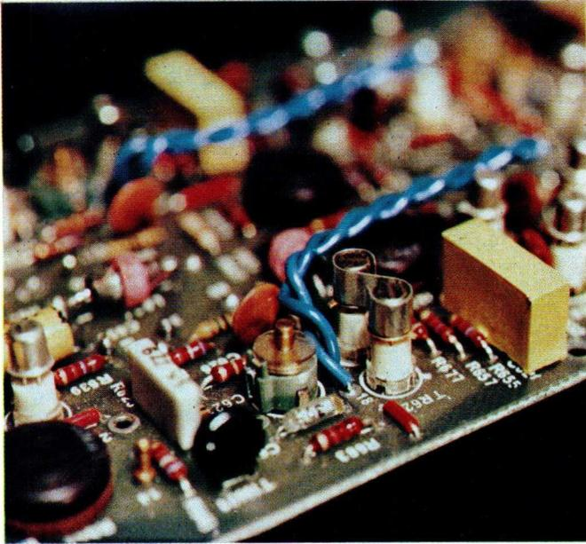
*Detail of the input stage of an oscilloscope showing a specially selected matched pair of n-channel FETs (similar to the BFS21/21A family) which are thermally coupled by means of a metal S-clip. (Photograph by courtesy of Telequipment Ltd, England).*
