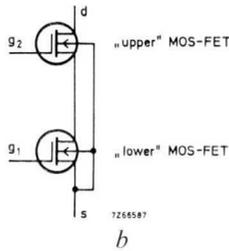
Fig.20 (a) Cross-section through MOS field-effect transistor with two gates (MOS-FET tetrode, see Plate D). (b) Circuit diagram of the MOS-FET shown in Fig. 20*a*.
