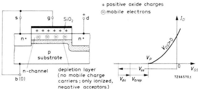
Fig.14 Elements of the pinch-off voltage  $V_p$  for a normally-on n-channel MOS-FET. A channel is already present at  $V_{GS} = 0$ . Normally-off n-channel types can be achieved by making  $V_{dc}$  high enough (high doping of the p-type substrate). The channel constriction at the drain end, caused by the drain current, is not shown here – drain current is assumed to be zero.
