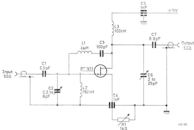
Fig.80 100 MHz common-source amplifier.
