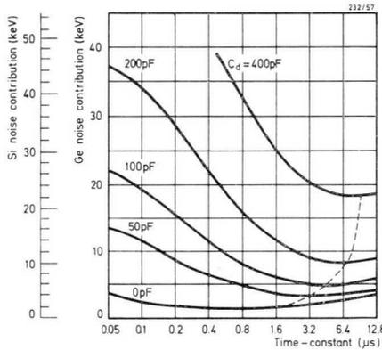
Fig.57 Noise contribution of pre-amplifier as a function of detector capacitance and amplifier time-constant.
