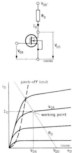
Fig.36 Fixing the operating point of junction and MOS field-effect transistors.
