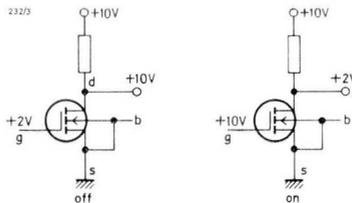
Fig.3 An inverter based on a MOS field-effect transistor (“normally-off” n-channel type; see section 3.2).
