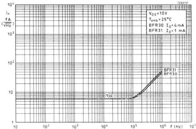
Fig.35 Equivalent noise current vs. frequency of a junction-FET.
