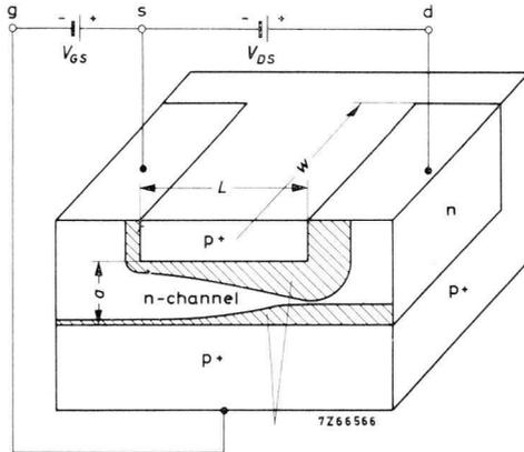
Fig.6 Schematic sectional view of a junction field-effect transistor (PN-FET), n-channel type. (The two p<sup>+</sup> regions – upper and lower gate – should also be imagined to be connected in front of the plane of the paper, so that the n-channel is in fact surrounded by an annular gate region).
