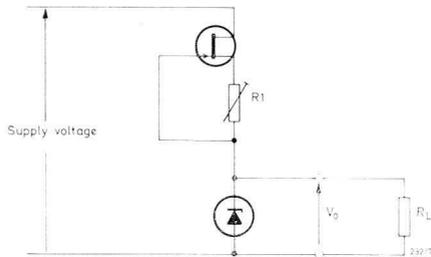
Fig.71 Stabilized current source for voltage reference diode.
