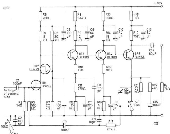
Fig.42 Camera pre-amplifier using cascaded BSV79 FETs in the input stage.
