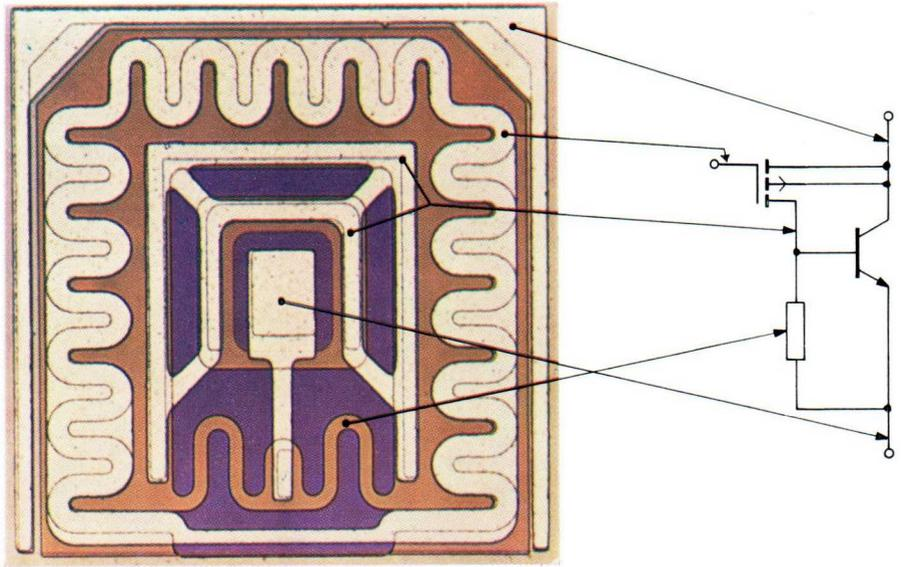
Plate E. Construction of the integrated circuit TAA320 comprising a p-channel enhancement MOS-FET, a bipolar transistor and a resistor.
