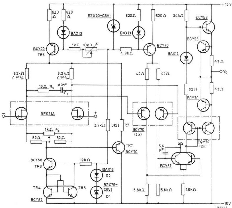
Fig.76 Circuit diagram of a high CMRR operational amplifier.
