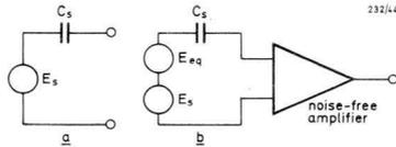
Fig. 44 Equivalent circuit of a capacitor microphone, (a) without, and (b) with noise voltage source due to an impedance matching network.
