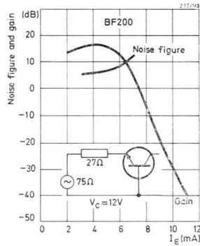
Fig.95 Noise figure and gain versus emitter current for BF200, plotted for comparison with Fig. 94.
