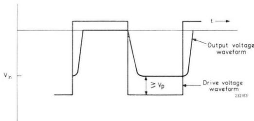
Fig.63 Switching waveform.
