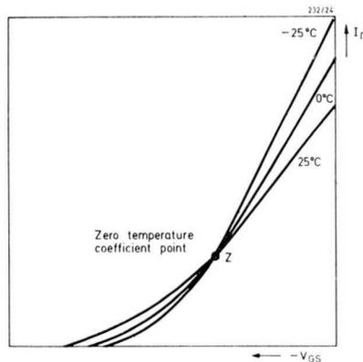
Fig.24 Temperature dependence of the  $I_D - V_{GS}$  characteristic of an n-channel field-effect transistor. The compensation point  $Z$  is subject to manufacturing spread of the pinch-off voltage.
