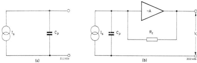
Fig.40 (a) Equivalent circuit of the output of the Plumbicon  $\text{\textcircled{R}}$  tube. (b) The camera pre-amplifier with feedback applied.
