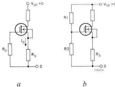
Fig.38 Stabilisation of the operating point of junction and MOS field-effect transistor by d.c. feedback with a source resistance  $R_S$  in combination with (a)  $R_G$  and (b)  $R_1/R_2$ .
