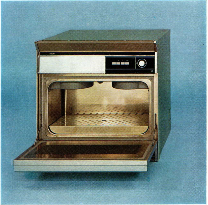
This 2.1 kW oven operates on 2.450 GHz and may be switched to operate at half power, if required. The oven walls are of stainless steel and the cavity dimensions are 505 mm (20") wide by 275 mm (11") deep by 220 mm (9") high. (By courtesy of Philips Domestic Appliances Division, Eindhoven, The Netherlands.)
