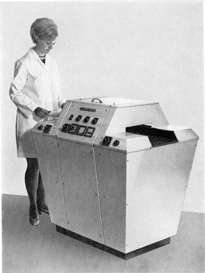
The 5 kW microwave oven described opposite, in which the moving belt oscillates back and forth. (By courtesy of Automatic Food Supplies Ltd., Växjö, Sweden.)
