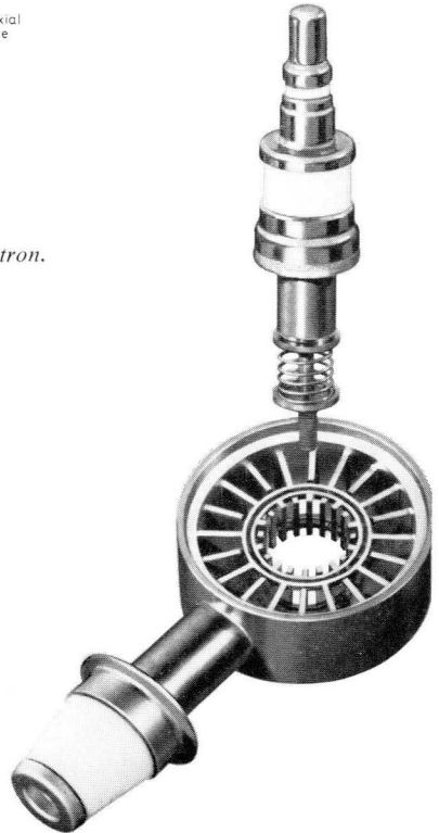
The cathode structure and the anode block of the 1/1.5 kW magnetron YJ 1280.
