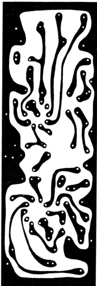
Fig. 4.13. Printed-wiring board for stereo version of one watt amplifier.
