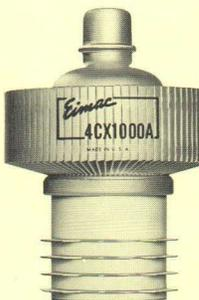
This high-power ceramic-metal tetrode is an excellent choice for applications where class-AB<sub>1</sub> operation is desired. It is capable of delivering more than 1500 watts plate output power per tube in audio or r-f service without requiring grid driving power. It is recommended for use in new equipments.
