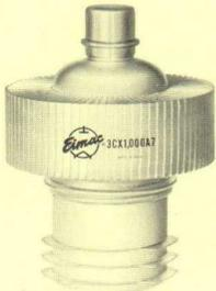
A new addition to the Eimac line of zero-bias triodes, the 3CX1000A7 features ceramic-metal construction and a mesh thoriated-tungsten filament. Positive socketing is provided by three breechblock terminal surfaces. This tube is intended for class-B linear amplifier service in either the grid-driven or cathode-driven connection. It is equally attractive for use at audio frequencies or at radio frequencies through the TV broadcast bands. It is recommended for use in new equipment.
