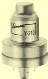
A special version of the ceramic and metal 4CX250B intended for use where small size and light weight are important. It may be cooled by liquid immersion or by the use of a suitable heat sink; maximum allowable plate dissipation is determined by the adequacy of the cooling provided but in no case should it exceed 250 watts.
