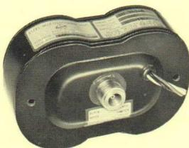
The X1089 and X1084 are nearly identical to the EM747 in construction and operation. They tune from 190 to 300 and from 300 to 600 Mc respectively with minimum power outputs of 20 and 30 mW. Ceramic-metal construction enables these tubes to survive extreme environments. Conduction cooling eliminates the need for cooling hardware. Temperature compensation for minimum frequency drift can be provided on special order.
