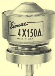
The veteran of external-anode tetrodes, and an Eimac original, continues to enjoy its deserved popularity. Recent tube improvements have made possible increases in maximum plate-voltage and plate-dissipation ratings. In Class-AB or Class-C service an input power of 500 watts is now allowed at frequencies up to 150 megacycles. The 4X150D is a 26.5 volt heater version of the 4X150A.
