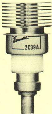
This old favorite among the many different UHF planar triodes is now supplied in an exclusive ceramic-and-metal envelope which assures higher efficiency and greater uniformity. The 2C39A is widely used as an oscillator, multiplier, or amplifier at frequencies up to 2500 megacycles. It is especially suitable for applications where performance requirements are not stringent or where economy is a major factor.
