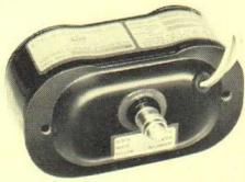
The X1085 voltage tunable magnetron weighs only 2 pounds, tunes from 1200 to 1400 Mc, and its ceramic-metal construction enables it to withstand severe missile environments. Normal power output is 100 mW with conduction cooling. A modified version, available on request, has a minimum power output of 1 W using forced air cooling. Specifications for the modified version are indicated below in **bold-face type**.
