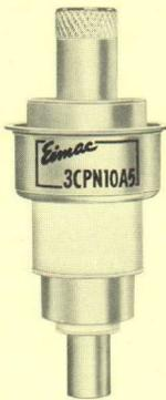
This ceramic and metal, UHF, planar triode is designed primarily for use in low-duty pulse applications. It is capable of delivering 1600 watts pulse output power at 3000 megacycles at a duty of 0.0025.
