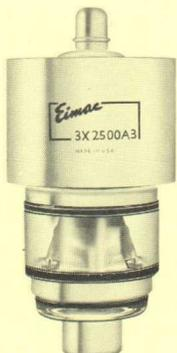
This popular high-power triode is widely employed in AM, FM, and TV service. Its coaxial filament and grid terminals insure low-inductance connection to these electrodes and allow operation at maximum ratings through 75 megacycles. The use of an external forced-air-cooled anode results in a compact structure with high power-handling capability.
