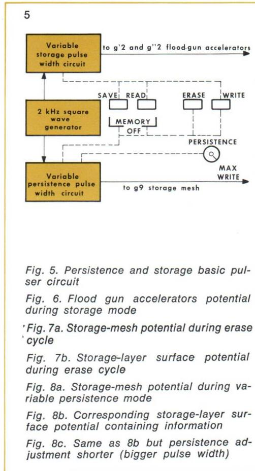
Fig. 5. Persistence and storage basic pulser circuit
