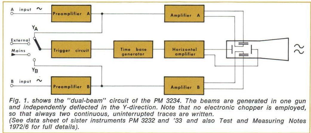
Fig. 1. shows the "dual-beam" circuit of the PM 3234. The beams are generated in one gun and independently deflected in the Y-direction. Note that no electronic chopper is employed, so that always two continuous, uninterrupted traces are written. (See data sheet of sister instruments PM 3232 and '33 and also Test and Measuring Notes 1972/6 for full details).
