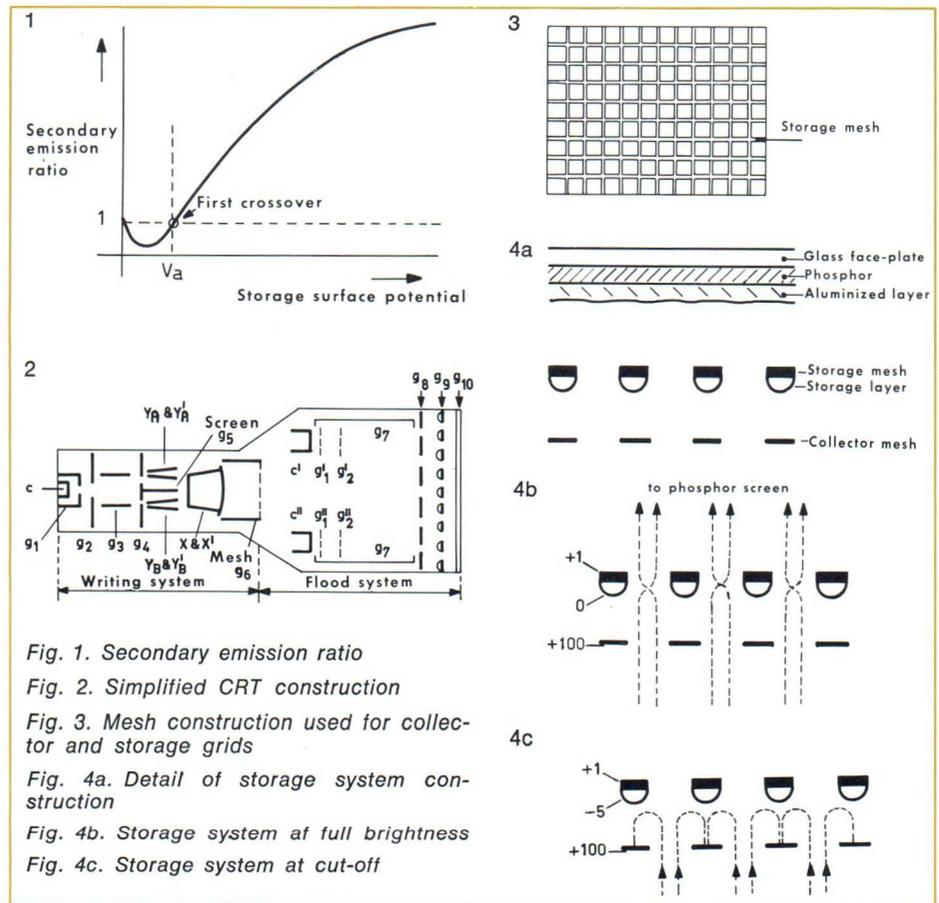
Fig. 1. Secondary emission ratio
