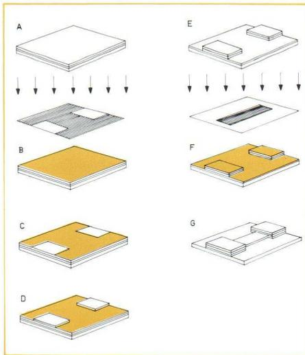
Fig. 2. The different steps in the production of a thin-film substrate.
