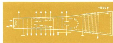
The combination of a very high acceleration voltage segmented vertical deflection plates, a special domed mesh after the deflection system and the big (8 x 10 cm) aluminized screen give a brighter, bigger display with an exceptionally high writing speed from a tube which is much shorter than normal.
