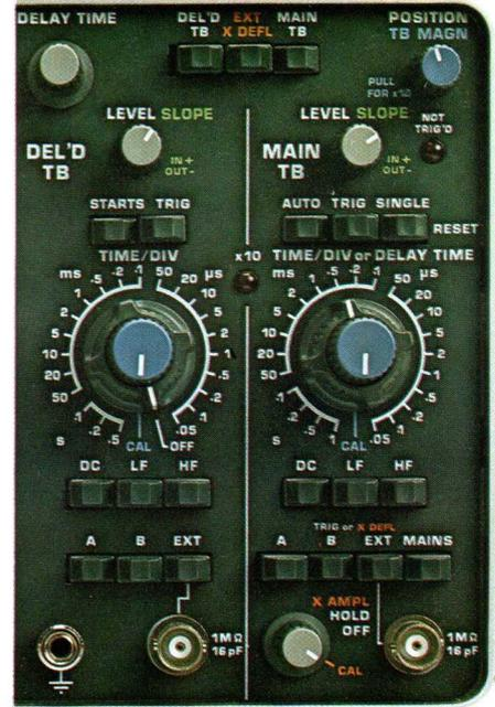
The main and delayed time base controls are separated in order to avoid ambiguity and possible errors. The controls are on the same level as those of the Y channels but clearly distinguishable. Note also that the vernier control of delay time is positioned so that the setting cannot be accidentally changed.
