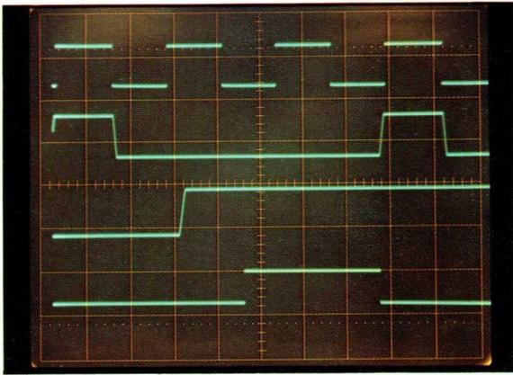
As illustrated, triggering is fully independent and multi-sourced. Main and delayed time bases can be triggered from any of the four signals plus Composite. The main time base can also be triggered on External and Line.
