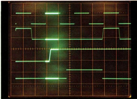
In this example the main time base is triggered on channel B and the delayed on channel A. It is therefore possible to magnify any delayed section of a signal in a stable manner even when it is not directly related to the main time reference.
