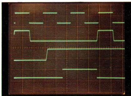
*In the PM 3244 four channel convenience is also combined with remarkable multi-source triggering. For example, main and delayed time bases can be triggered from many different signal sources.*
