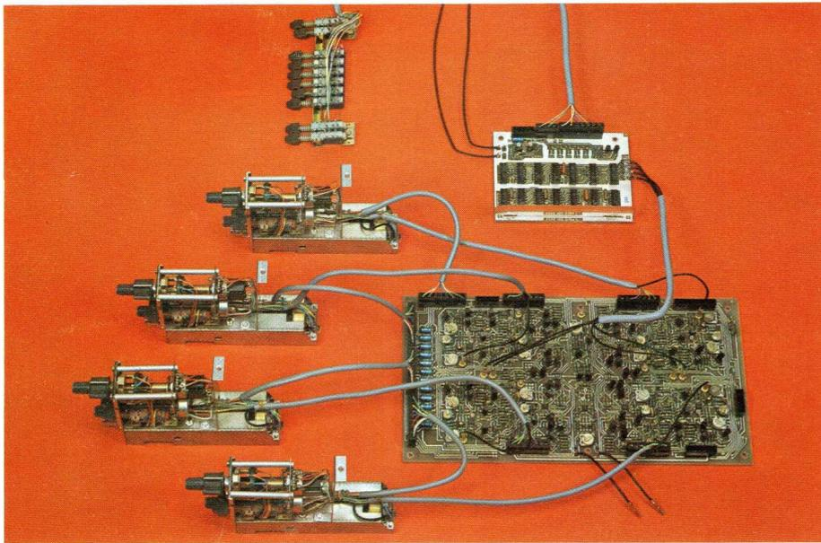
The main amplifier panel of the PM 3244 is electrically connected to front panel controls and simple DC signals are used to change operating parameters.
