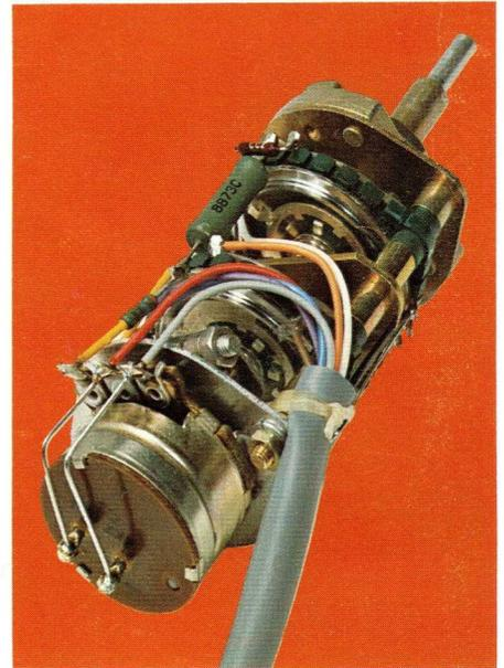
A dramatic simplification of the main time base switch as a result of cold switching techniques.
