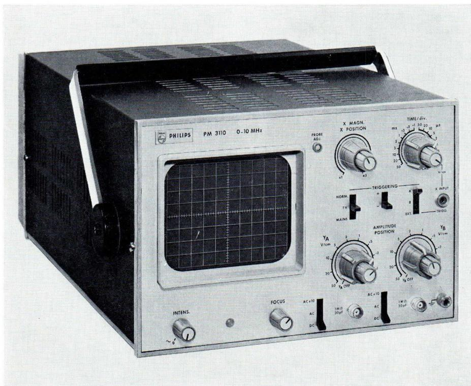
Fully automatic triggering, including TV line and frame
