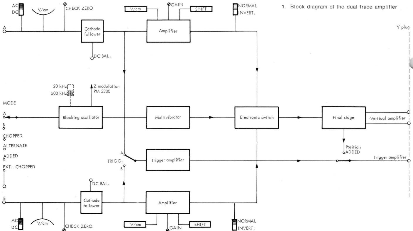
1. Block diagram of the dual trace amplifier
