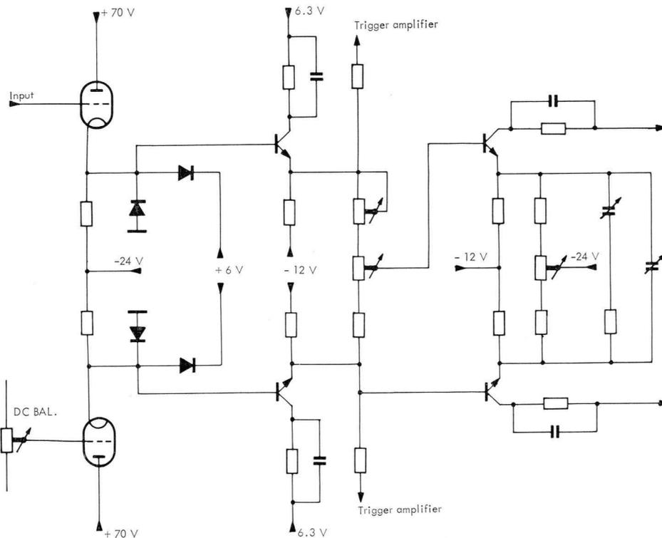
3. Circuit diagram of electronic switch
