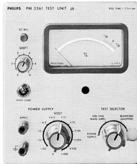
This plug-in facilitates testing of the main frame, output amplifier, power unit and blanking circuit. It provides:
