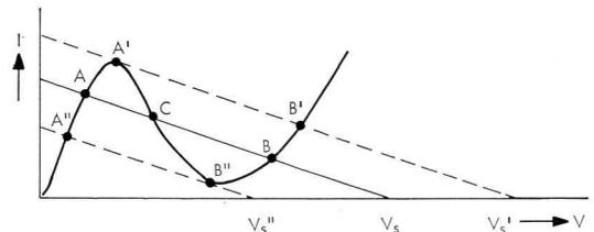
19. Characteristic of the tunnel diode with different load lines
