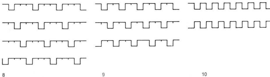
8. Waveforms on the collectors during the switching
