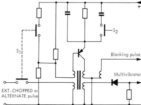
5. Circuit diagram of blocking oscillator
