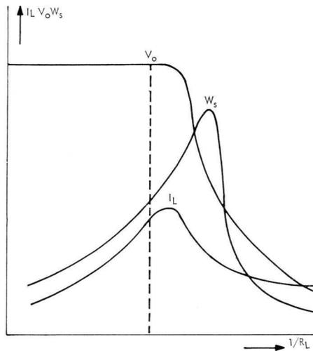
14.  $V_o$ ,  $I_L$  and  $W_s$  as a function of  $1/R_L$
