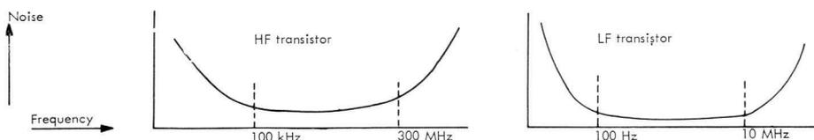
2. Noise frequency curves for HF and LF transistor
