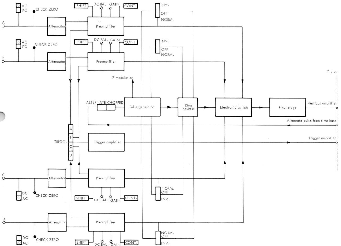
1. Block diagram of the four trace amplifier
