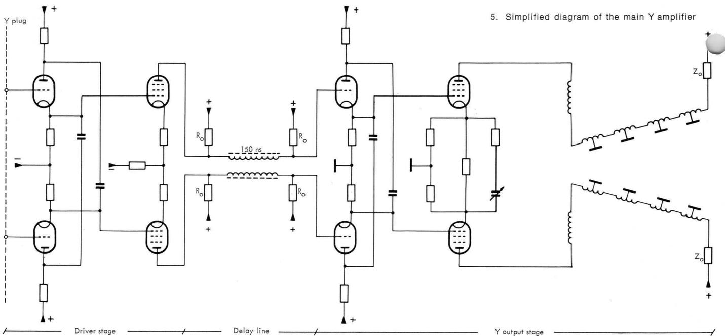
The input impedance  $Z_i$  then equals  $R_0$ , thus  $Z_i$  is independent of frequency.
