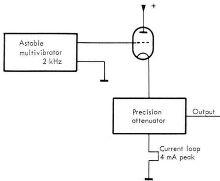
16. Simplified diagram of the calibration unit
