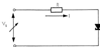
18. Simple tunnel diode circuit
