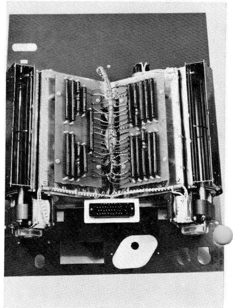
Cooling unit, with power transistors, can be taken out and interconnected with the apparatus by means of a connector block. The transistors on this cooling unit are then interchangeable. Special holder for the transistors renders soldering unnecessary
