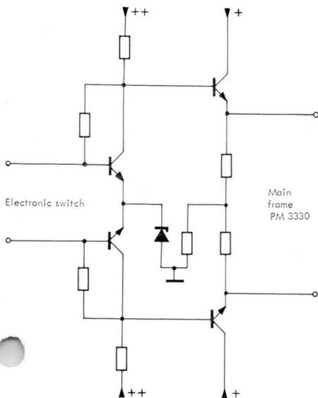
4. Circuit diagram of the final stage
