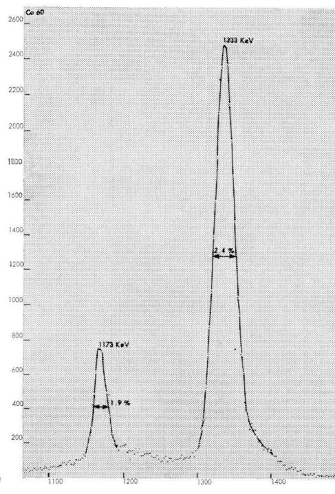
3. Co<sup>60</sup> spectrum recorded with the pairspectrometer described in this article
