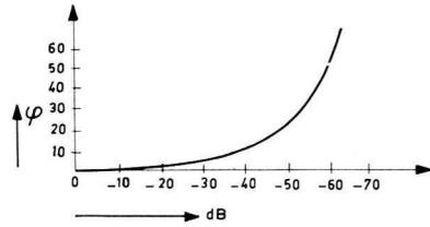
4. Phase difference  $\varphi$  as a function of attenuation
