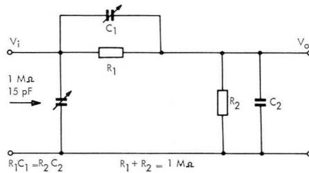
ductance of the capacitors and the earth connections, begin to play a role. In this way the attenuation becomes dependent on the frequency which, in pulse reproduction leads to distortion of the flanks. A great deal of care has therefore been devoted to the attenuator used in the PM 3333, with respect to good high-frequency earthing, and special HF disc capacitors of very low self-inductance have been incorporated.
