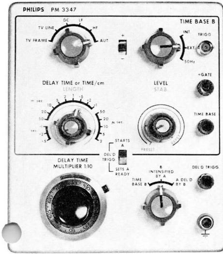
With the unit PM 3347 the oscilloscope is capable of displaying any small part of a signal which is complex with respect to time. Moreover accurate time interval and jitter measurements are possible. This unit can supply both a sawtooth voltage for the horizontal deflection and a trigger pulse for delayed starting time base generator A of the basic oscilloscope. Fig. 1 shows the block diagram of the unit and fig. 2 the relevant waveforms.
