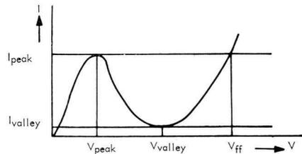
17. Tunnel diode characteristic
