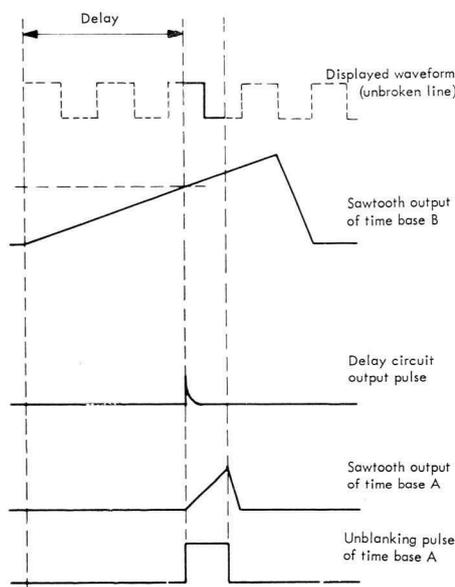
8. Waveforms obtained in operation with the gated working of A DEL'D BY B
