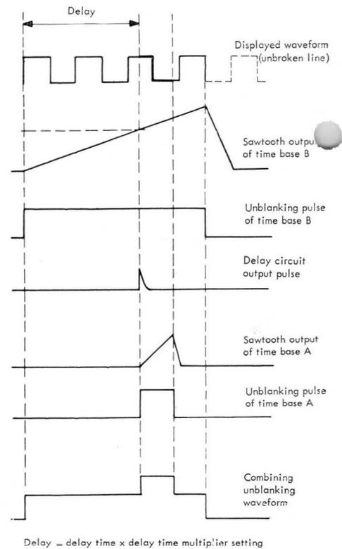
**Mode selector switch set to A DEL'D BY B**
