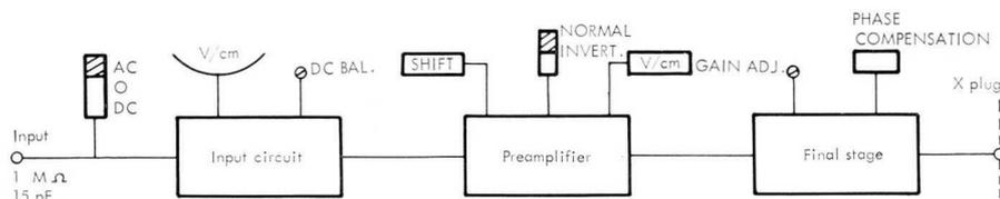
1. Block diagram of the horizontal amplifier
