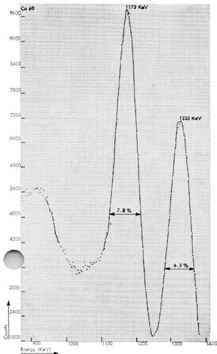
2. Co<sup>60</sup> spectrum recorded with a conventional single crystal spectrometer consisting of a 1<sup>3</sup>/<sub>4</sub>" diameter x 2" thick NaI (Tl) crystal coupled to a 2" photomultiplier tube
