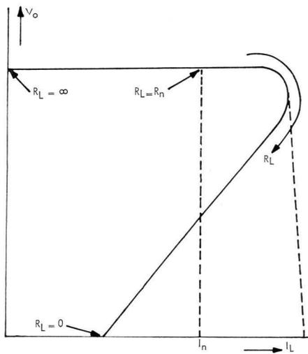
13. Output voltage as a function of the output current with parameter  $R_L$
