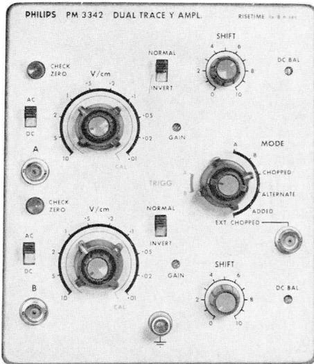
The PM 3342 is a plug-in preamplifier for the basic oscilloscope PM 3330 with two independent input channels (dual trace unit). The signal from either channel can be displayed individually or the two signals can be displayed simultaneously, either on a time-sharing basis (A and B) or algebraically added. Internal triggering is possible in both cases without the switching frequency causing any hindrance.
