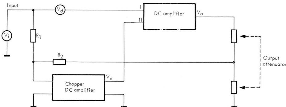
1. Simplified diagram of the chopper stabilization
