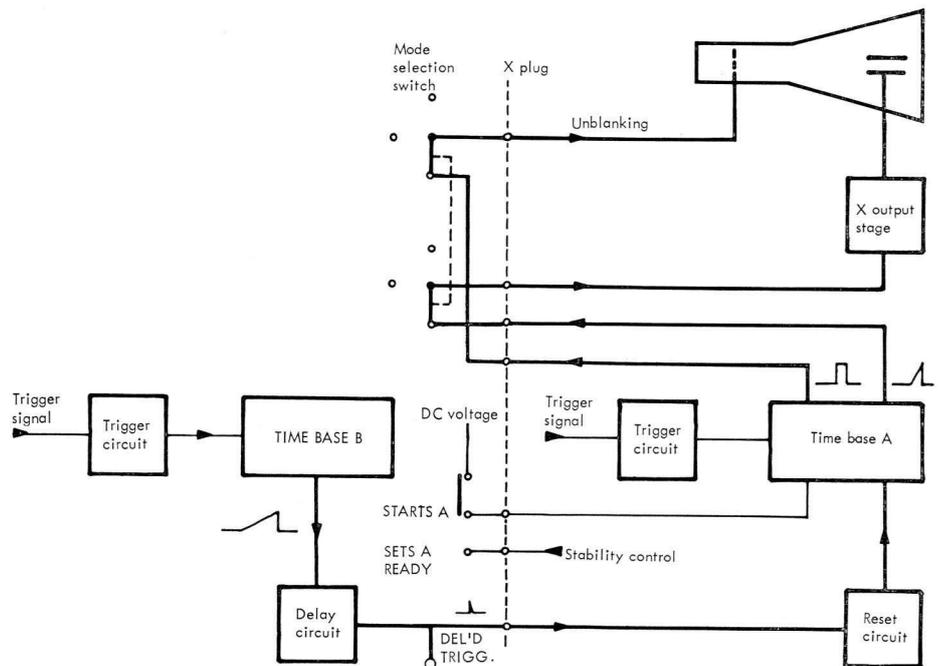
6. Mode selector switch set to A DEL'D BY B
