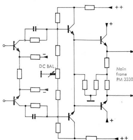
5. Circuit diagram of trigger amplifier
