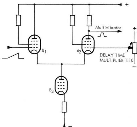
9. Voltage comparator circuit
