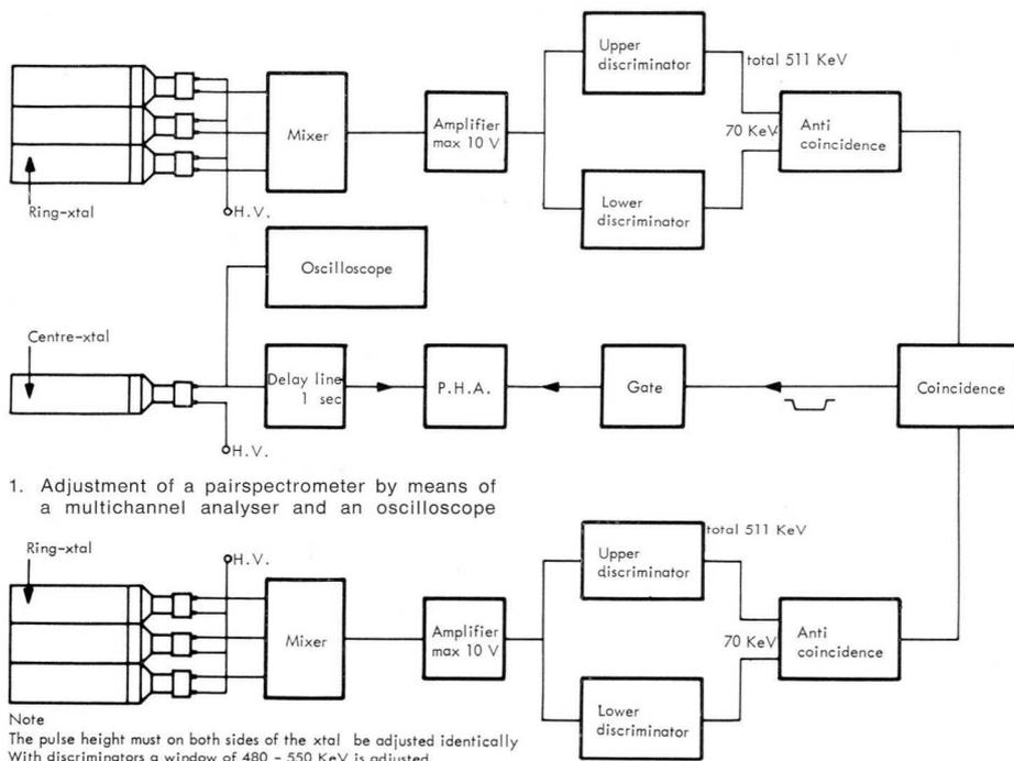
1. Adjustment of a pairspectrometer by means of a multichannel analyser and an oscilloscope
