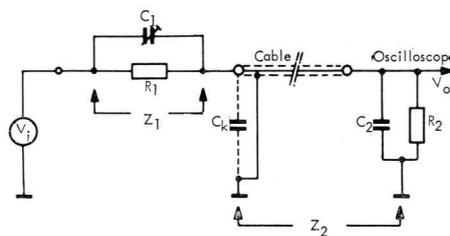
5. Principle of the passive probe
