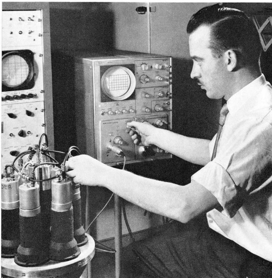
A special gamma radiation spectrometer is described, which has several advantages over the conventional single crystal spectrometer. These advantages are:
