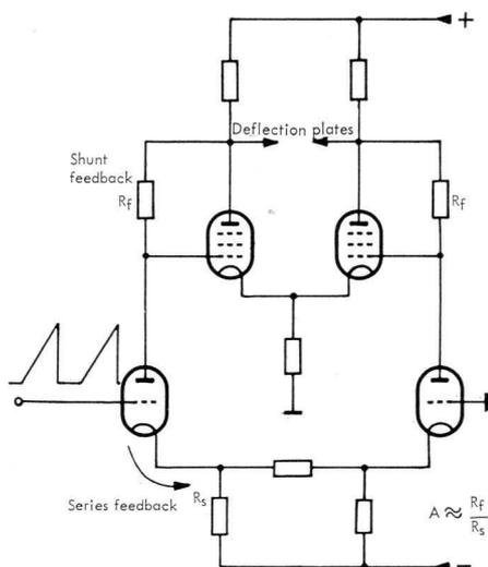
9. Parphase amplifier as used in the X output stage
