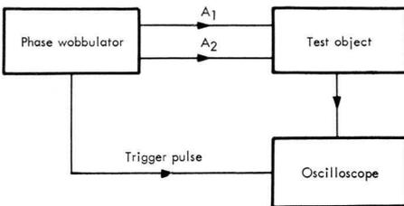
The output voltage of this circuit depends on phase angle  $\varphi$ . If it is required to measure the output voltage, represented on the vertical axis of the oscilloscope, as a function of phase angle  $\varphi$  of the input voltage, the horizontal axis of the oscilloscope must be calibrated as a function of  $\varphi$ . The scale of  $\varphi$  is linear so that the
