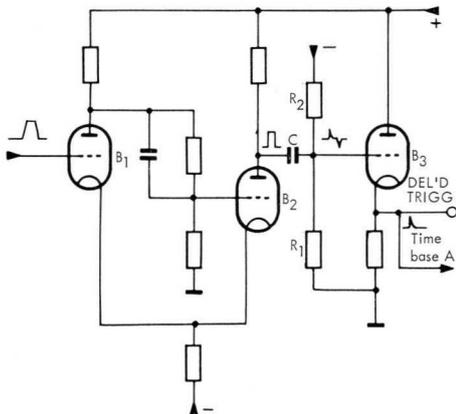
10. Pulse shaper and its associated circuits
