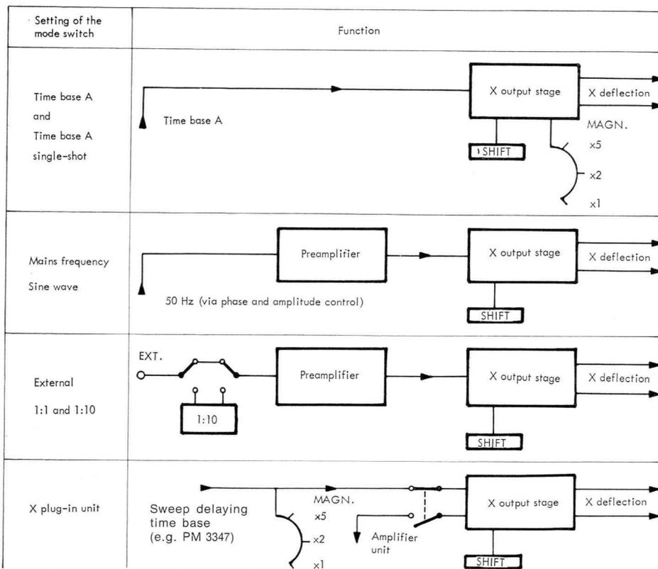
8. Survey of functions of the horizontal amplifier circuit
