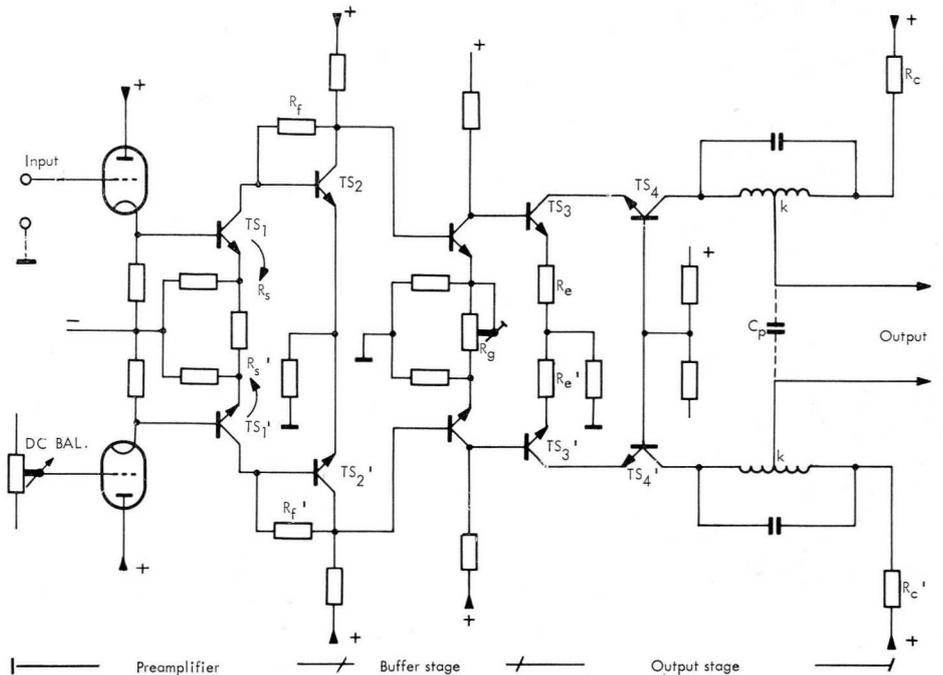
Because of this and the low output resistance of  $TS_2$  the preamplifier stage has a wide bandwidth. For a detailed treatment of this circuit, reference is made to the articles written by Dr. Cherry and Mr. Hooper, of the Department of Electrical Engineering, University of Melbourne.\*
