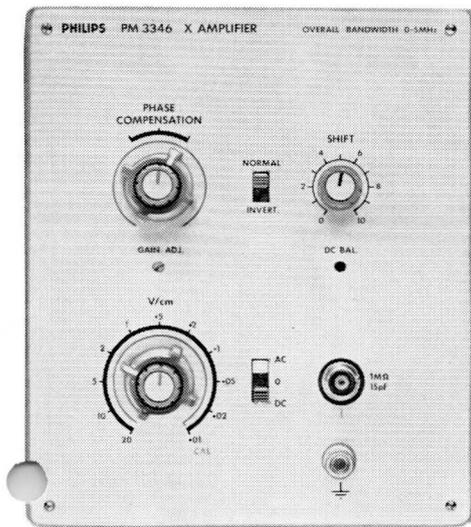
The PM 3346 is a plug-in unit designed for the horizontal channel of the PM 3330. This unit enables the PM 3330 to be used as an X-Y oscilloscope, fig. 1.
