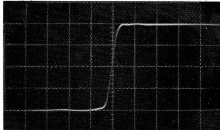
4. Overall step response of the amplifier; rise time of the input signal amounts to about 1ns, time scale 10 ns/cm
