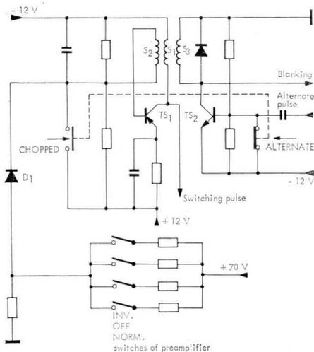
6. Circuit diagram of the pulse generator containing the blocking oscillator and pulse shaper
