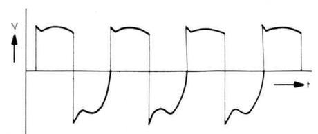
20. The voltage across a tunnel diode with sine-wave input
