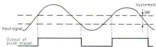
5. Indicates the levels of the input signal at the point where the pulse shaper switches on and off, due to the "hysteresis gap" at the input of the pulse shaper. The figure shows how triggering occurs when the trigger level selector is in position "MEAN"; the mean value of the input signal is near by or with in the hysteresis gap
