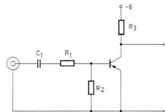
3. Basic circuit arrangement of a pulse shaper for line pulses
