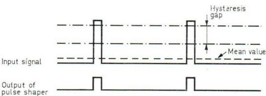
6b. Trigger level selector in position "TOP". Due to top detection and DC restoring the "hysteresis gap" is shifted towards the top value of the input signal. The pulse shaper can now be switched; and the time base can be triggered nearby the top value of the input signal
