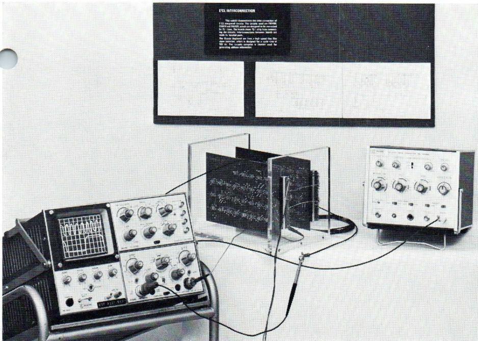
3. Testing of E<sup>2</sup>CL circuits with PM 5770
