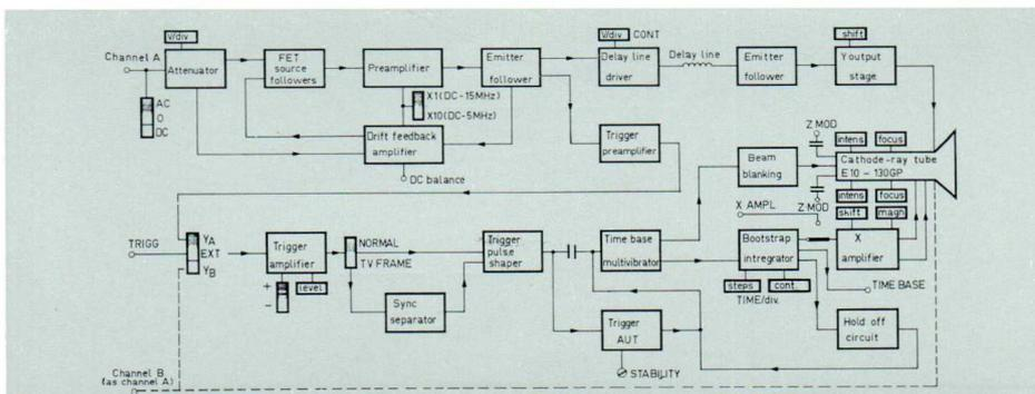
Rapid increase in the application of digital techniques has created a demand for economical and simply operated double-beam oscilloscopes permitting accurate measurement and comparison of the shape, amplitude, rise time, repetition frequency, etc. of pulses. This new double-beam oscilloscope will assist in meeting this demand. Block diagram is shown in fig. 1. The main features of the PM 3231 oscilloscope are:
