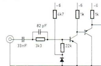
5. Complete diagram of the pulse shaper is shown here
