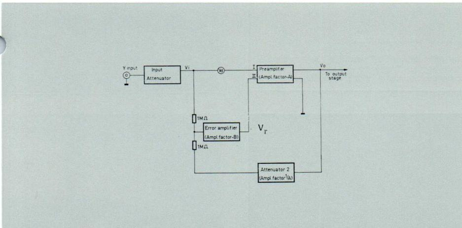
2. Simplified block diagram of drift compensation circuit
