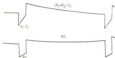
6a. Same circuit given in fig. 3 is not advisable to be used for frame pulse because of the difficulty to separate this frame pulse from superimposed hum
