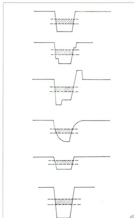
1. Examples of TV pulses distorted by the cable distribution network due to reflections, wrong terminations, cable losses etc.
