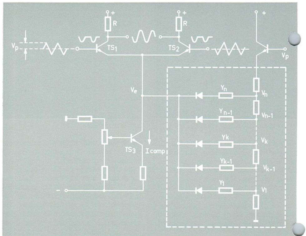
Basic circuit of triangle - sine converter
