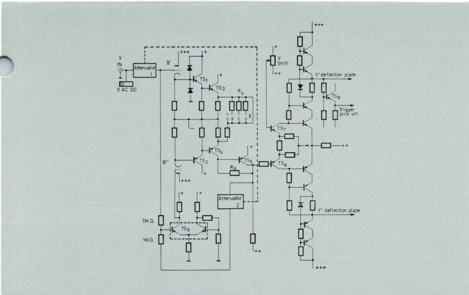
1. Vertical deflection system showing preamplifier, drift compensation circuit, output stage and trigger pick-off
