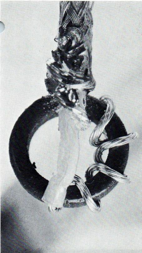
of making such a transformer is to use a ferroxcube toroid (Philips 2 P 65331). The collector current is fed through the hole of the toroid forming a one turn primary winding. The secondary winding can be made in the following way. Use a standard teflon 50 Ω coaxial cable (as RG 188). Strip off the screening and the outer cover but leave approx 5 cm of the inner conductor. This wire is wound 5 turns around the toroid and soldered to the cable screen. Fig. 3 shows how the transformer is added
