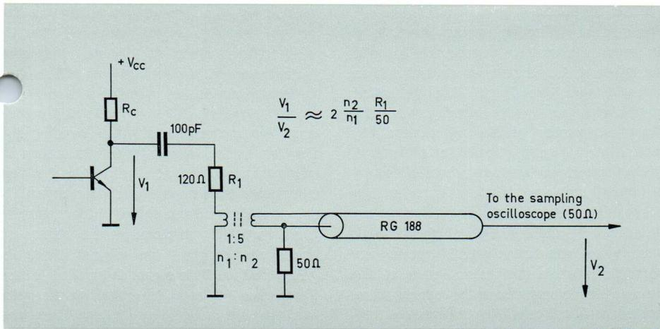
3. Current transformers can be applied for nanosecond phenomena. The figure shows the schematic diagram for an inductive probe and how it can be connected in the same electronic circuit, as in fig. 1
