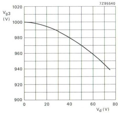
Fig. 6 Focusing voltage (V<sub>g3</sub>) as a function of grid drive voltage (V<sub>d</sub>); typical curve.
