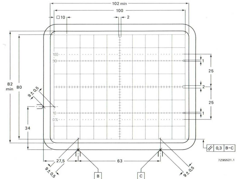
Fig. 5 Front view of tube with internal graticule, type 123 (final accelerator contact at left-hand side). The faceplate reference points are used for aligning the graticule with the faceplate.
