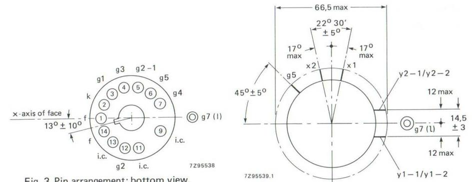
Fig. 3 Pin arrangement; bottom view.
