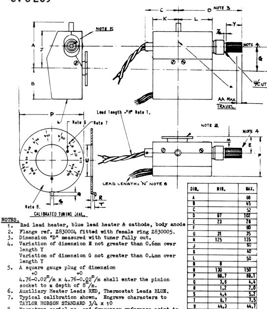
8. Magnetron serial no. and frequency reference point to be engraved on reverse s ide as follows:-Serial Number \* For \* Gc/s Set \* On micrometer Dial.
