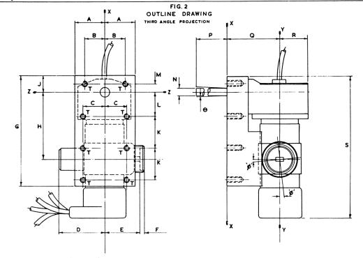
Waveguide output mates with a standard Interservice Coupler Lecating Ring Ref Z830017 and Ring Nut Ref Z930020 to W.G.22
