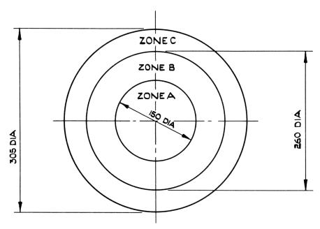
ZONE 'C' EXTENDS OVER EDGE OF SCREEN DOWN TO MOULD MATCH LINE. SCREEN WALLS EXTEND FROM MOULD MATCH LINE TO WELD LINE.
