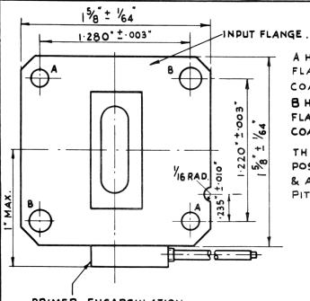
A HOLES - 2 HOLES IN EACH FLANGE · 150"DIA ± · 002" COAXIAL TO EACH OTHER. B HOLES - 2 HOLES IN EACH FLANGE · 170"DIA ± · 002" COAXIAL TO EACH OTHER.
