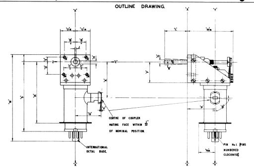
THE VALVE IS DESIGNED FOR USE WITH A FLOATING BASE SOCKET & NO UNDUE STRAIN SHOULD BE PUT ON THE OUTPUT COUPLER.
