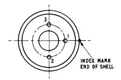
INPUT CHOKE SPIGOT, INDEX MARK & PIN No.! WILL NOT DEVIATE FROM A COMMON & BY MORE THAN 15° IN EITHER DIRECTION
