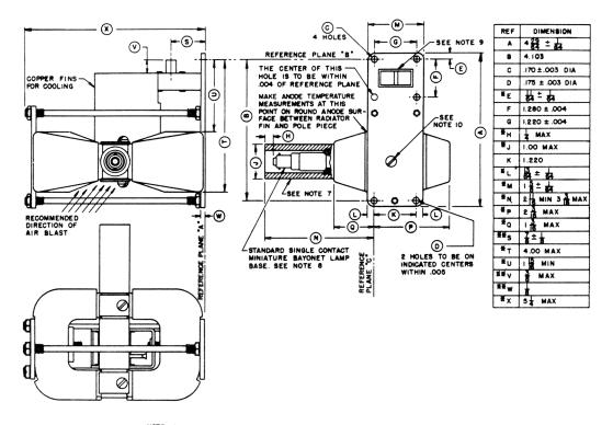
NOTE 1: REFERENCE PLANE "B" PASSES THROUGH THE CENTERS OF THE TWO TOP HOLES OF THE MOUNTING PLATE AS SHOWN AND IS PERPENDICULAR TO PLANE "A" NOTE 2:
