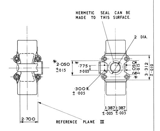
FOR FURTHER DIMENSIONS & INFORMATION SEE SPEC. MIL - E- I / 979 C. ON SPEC. MIL - E- I / 979 C DIMNS. B & C ARE REDUNDANT, DIMNS. H & AU ARE REPLACED.
