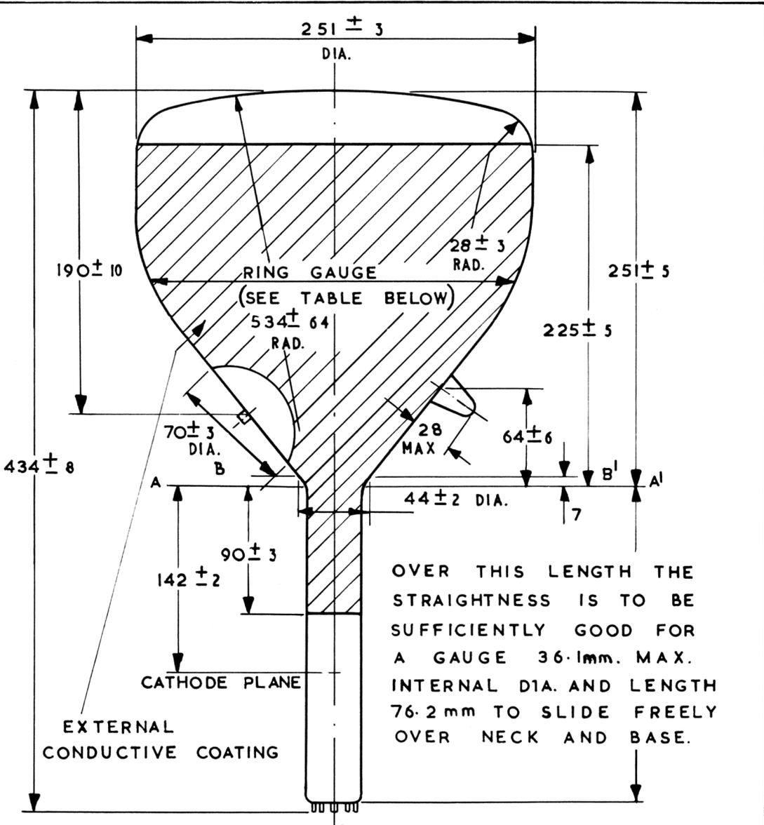
OVER THIS LENGTH THE STRAIGHTNESS IS TO BE SUFFICIENTLY GOOD FOR A GAUGE 36.1mm. MAX. INTERNAL DIA. AND LENGTH 76.2 mm TO SLIDE FREELY OVER NECK AND BASE.
