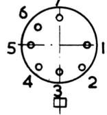
A2 AND EXHAUST PIP TO BE WITHIN  $\pm 15^\circ$  OF LINE THROUGH PINS 3 AND 7 OF BASE.
