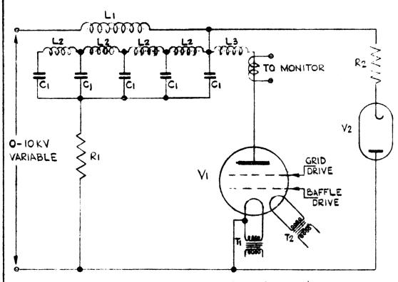
VI = CV V2 = SUITABLE REVERSE DIODE Zo = 12.85 \( \Omega\) PULSE LENGTH = 1.8 \( \Omega\) SEC. PR.F. = 800 CYCLES. MEAN CURRENT = 1 AMP. RATE OF RISE = 5,000 A/\( \Omega\) SEC. HOLD OFF VOLTAGE = 18 KV. PEAK CURRENT = 700 AMPS. RI = 12.85 \( \Omega \frac{1}{2} \) \( \Omega \)
