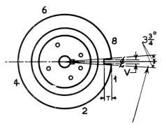
RING KEYWAY & BASE KEY SHALL NOT DEVIATE FROM A COMMON & BY MORE THAN 3 3/4 IN EITHER DIRECTION.
