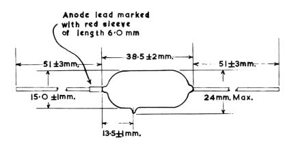
Leads shall be flexible and tinned to a length of at least 38mm
