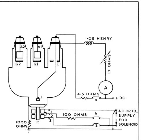
AI-LOW VOLTAGE ANODE. GI-LOW VOLTAGE GRID. A2-HIGH VOLTAGE ANODE. G2-HIGH VOLTAGE GRID. EI- EXCITATION ANODE.
