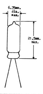
SPACING OF LEADS 1.5 nm. Min. THE LEADS SHALL BE TIRRED FLEXIBLE 25-29 S.W.G. WIRE, AT LEAST 15.0 mm. IN LENGTH.
