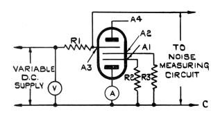
V = VOLTMETER A = LOW RESISTANCE MILLIAMMETER RI = 2.3K R2 = .25 M.
