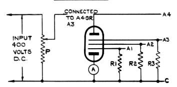
P = POTENTIOMETER. A = LOW RESISTANCE MILLIAMMETER. RI = R2 = R3 = .25 M
