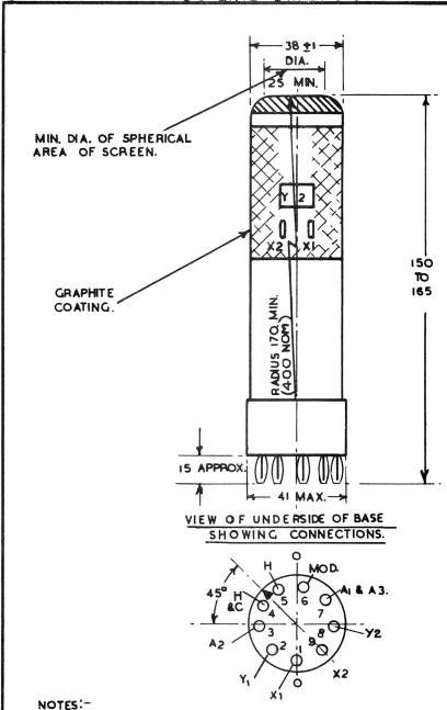
L. VIEWING THE SCREEN OF THE TUBE WITH THE BASE ORIENTATED AS SHOWN ABOVE, A POSITIVE POTENTIAL APPLIED TO PIN No. (XI) SHALL DEFLECT THE SPOT TO THE LEFT AND A POSITIVE POTENTIAL APPLIED TO PIN No. 2 (YI.) SHALL DEFLECT THE
