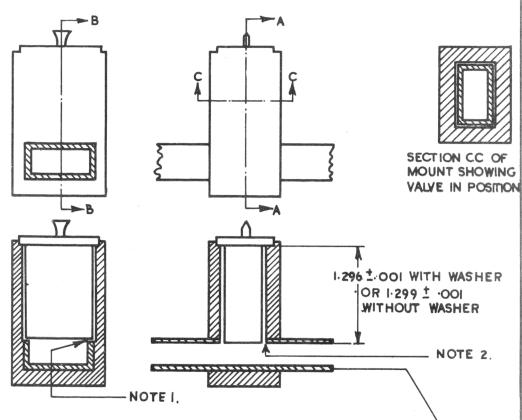
SECTION AA OF MOUNT SHOWING VALVE IN POSITION. SECTION BB OF MOUNT SHOWING VALVE IN POSITION. PIECE OF STRAIGHT WAVEGUIDE OF INTERNAL DIMENSIONS 0.4 BY 0.9.
