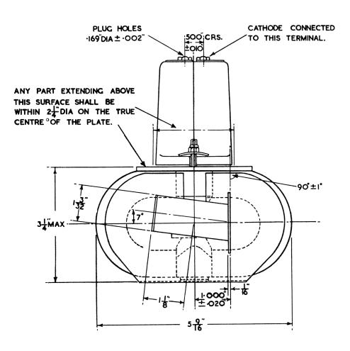
THE NORTH POLE OF THE MAGNET SHALL BE ADJACENT TO THE MOUNTING FLANGE.
