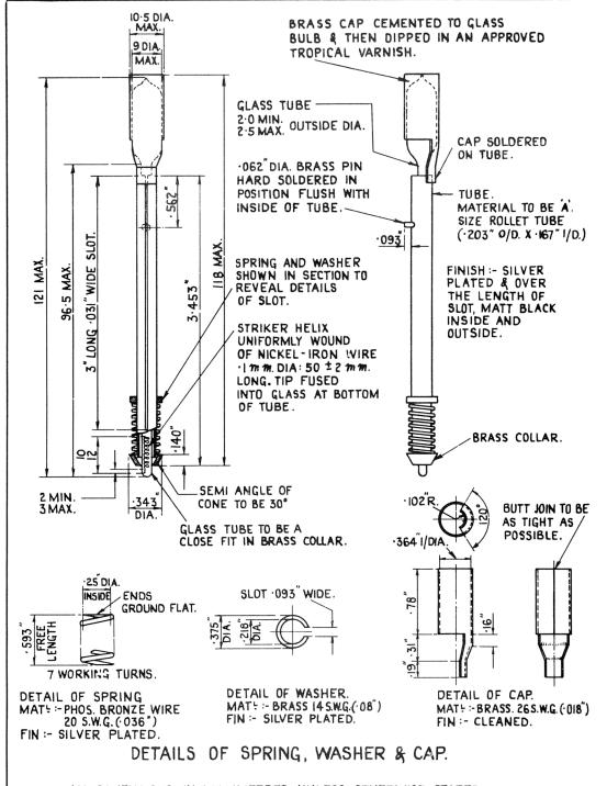
ALL DIMENSIONS IN MILLIMETRES UNLESS OTHERWISE STATED. TOLERANCE ON ALL INCH DIMENSIONS TO BE  $^\pm \cdot 005$  "
