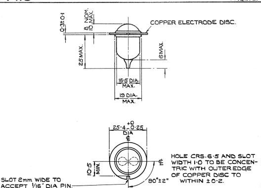
DETAIL OF HOLE PUNCHED OUT OF COPPER DISC.
