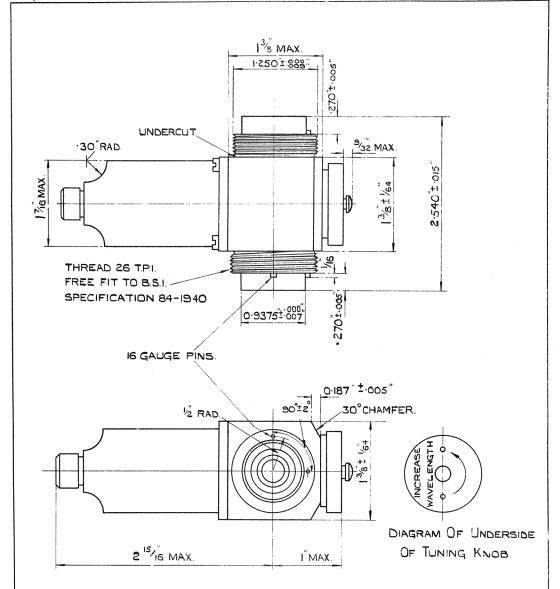
APPRECIABLE DEVIATION FROM THE OUTLINE OF BLOCK SHEWN ABOVE IS PERMISSIBLE PROVIDED DIMENSIONAL TOLERANCES ARE NOT EXCEEDED.
