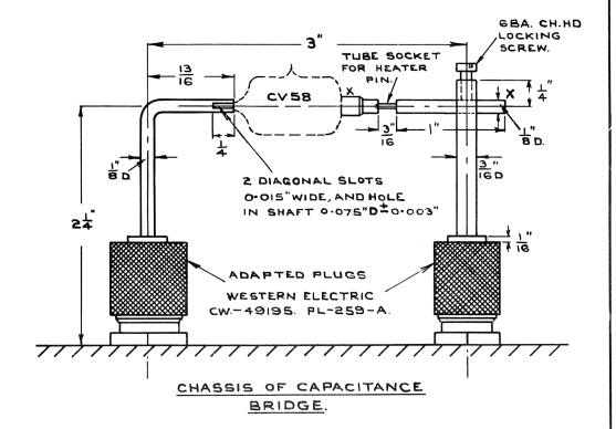
NOTE, D.C. HEATER VOLTAGE TO BE APPLIED BY CLIPPING FLEXIBLE LEADS ON TO POINTS XX.
