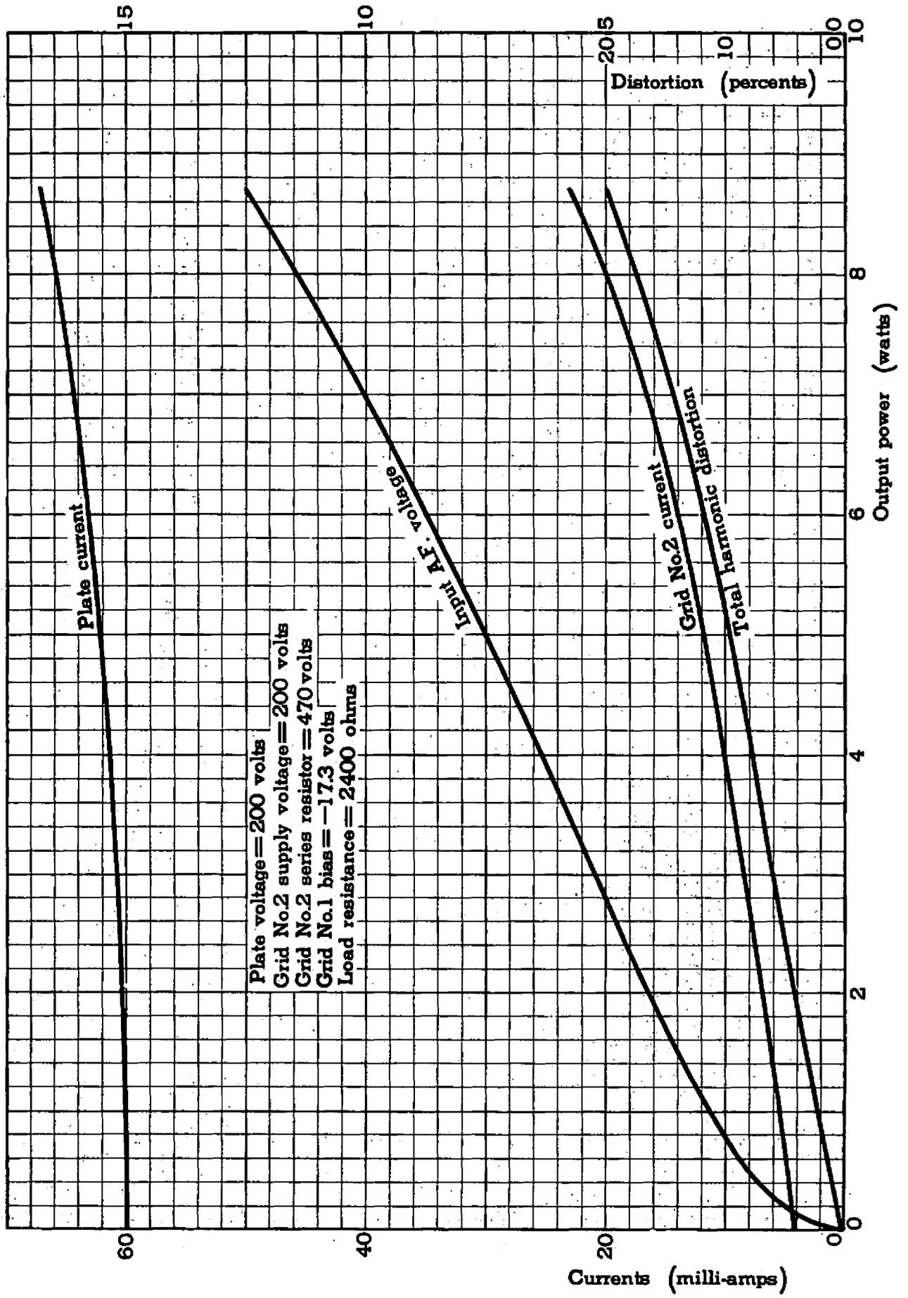
Input A.F. voltage (volts, RMS.)
