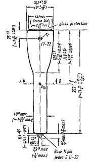
The tube must not be mechanically stressed when attaching or removing the socket.
