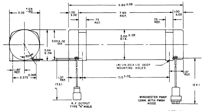
A-COLLECTOR B-HELIX C-HEATER D-HEATER, CATHODE E-ANODE F-GRID (FOCUS)
